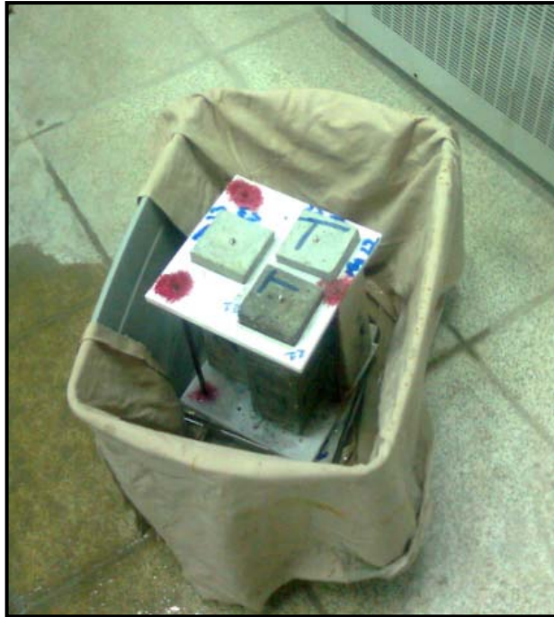
Figure 6. The ASTM C 1293 Testing Setup – Open View
