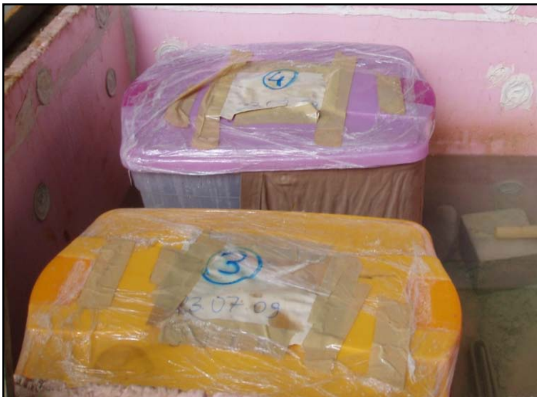
Figure 7. The ASTM C 1293 Testing Setup – Sealed View
