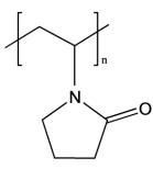
**Figure 2** Structure of poly(N-vinyl-2-pyrrolidone)
