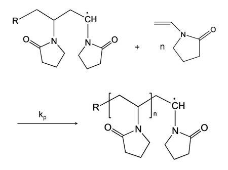
Figure 5 Growth of the polymer chain
