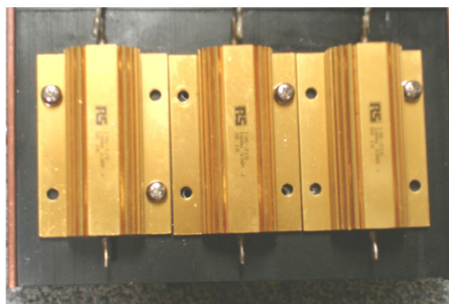
Figure 4.27 Precharge Resistors fixed to Heatsink
