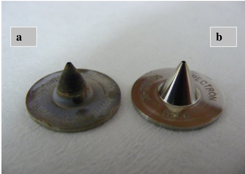
Figure 3. 30 Skimmer cones with (a) and without (b) C deposition
