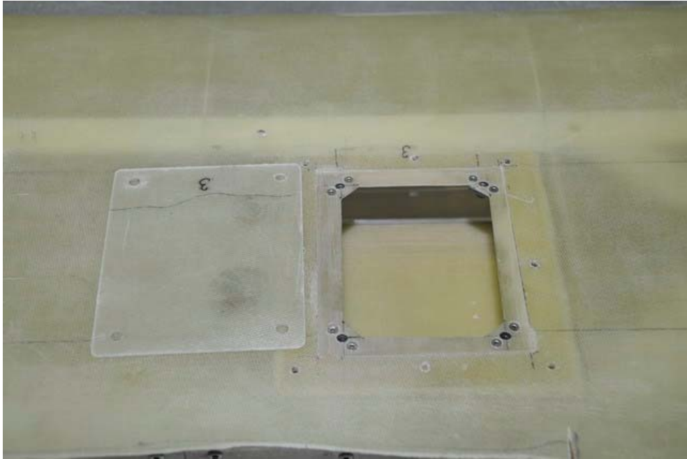
Figure 56: Servo Motor Access Seal and the Support Structure on the Composite Skin
