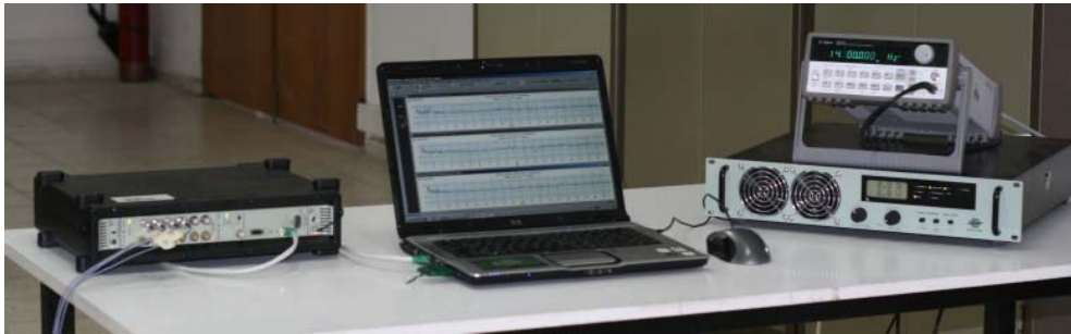
Figure 63: The Control and Analyses Equipments Used in Ground Vibration Tests (From Left to Right, FFT Analyzer, Computer, Signal Generator at top and Power Amplifier at bottom)
