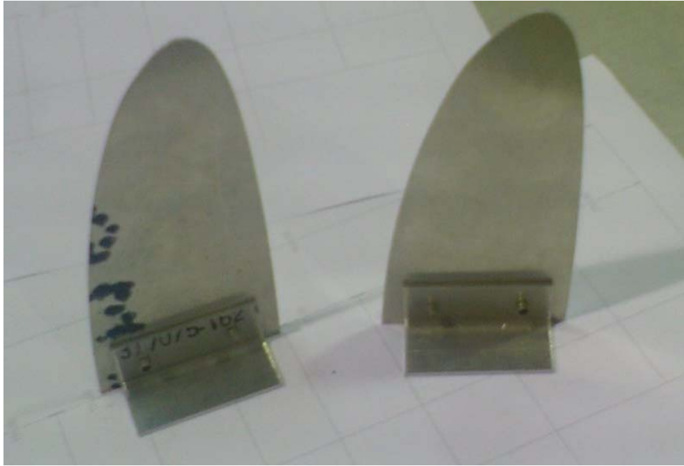
Figure 52: Assembly of Leading Edge Rib Portions and Corner Connectors by ST3210 Steel Rivets
