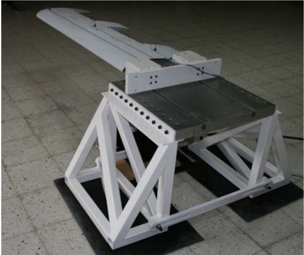
Figure 105: The Picture of the Assembled Vibration Test Bench and the Wing Torque Box Mounted on It
