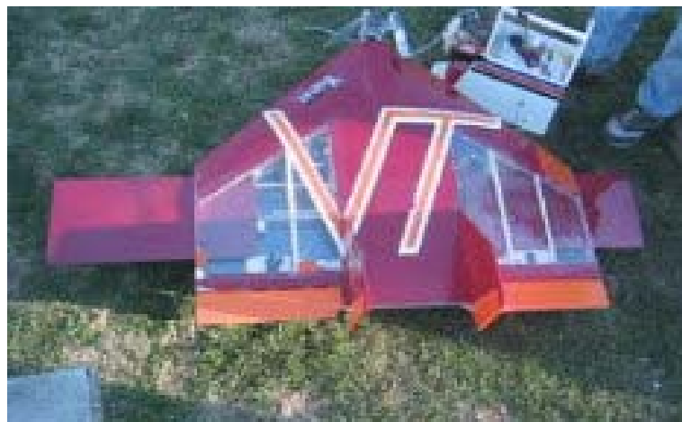
Figure 2: Anti-symmetric Wing Extension Mechanism [3]
