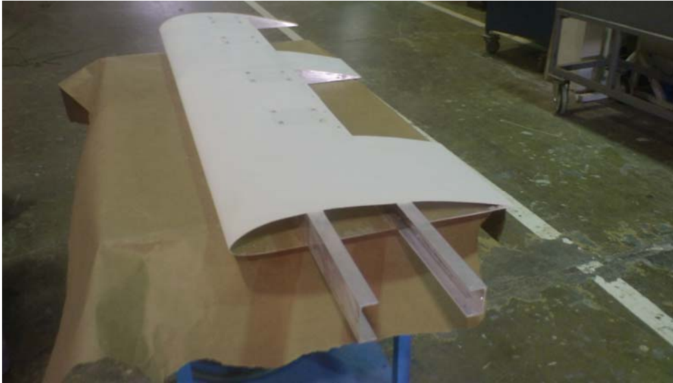
Figure 59: The Assembled Wing Torque Box Structure
