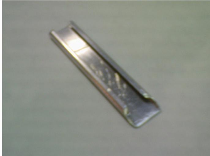
Figure 4.15: Track of the Guide-Slide Assembly
