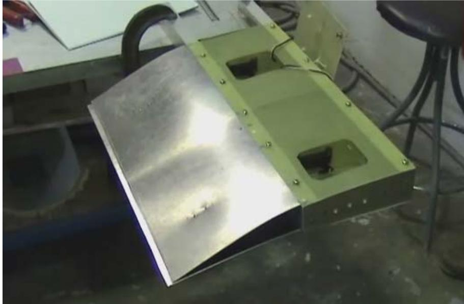
Figure 4.19: Hingeless Control Surface with Constant Positive Chordwise Actuation
