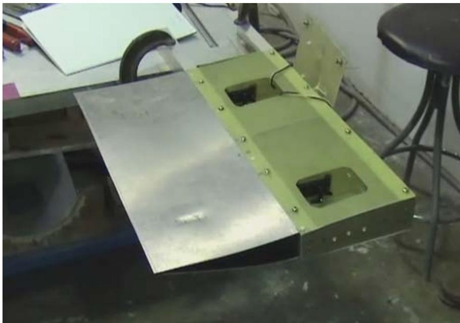
Figure 4.20: Hingeless Control Surface with Constant Negative Chordwise Actuation
