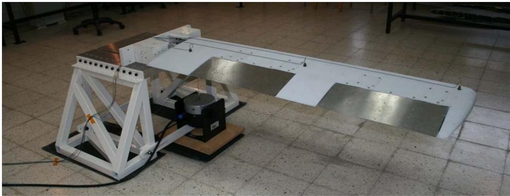
Figure 4.39: Adaptive Camber Wing Attached to Fixture, Modal Shaker and Accelerometers Attached to the Wing
