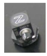
Figure A.2 3-axial piezoelectric accelerometer
