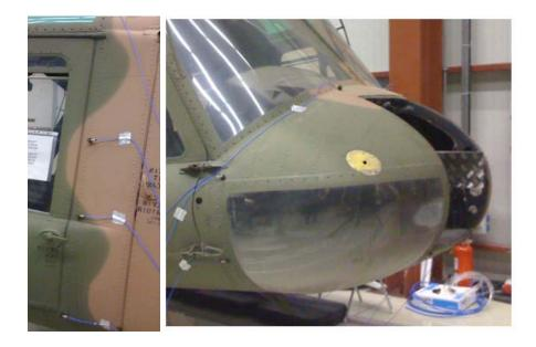
Figure 5.10 Accelerometer locations at main body front
