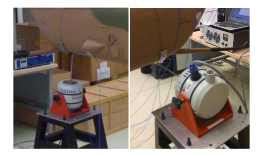
Figure 5.13 Stinger directions, vertical and transverse respectively
