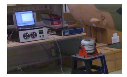
Figure 5.11 Shaker, controller, and amplifier system
