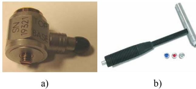
**Figure 3.5 a) Force Transducer, b) Impact Hammer with different tips**
