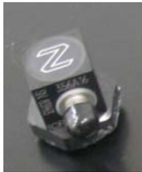
**Figure A.2 3-axial piezoelectric accelerometer**
