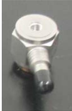
**Figure A.3 Single axis force transducer**
