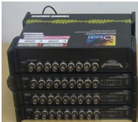
**Figure A.1 Iotech data acquisition system**
