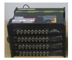
Figure A.1 IOtech data acquisition system
