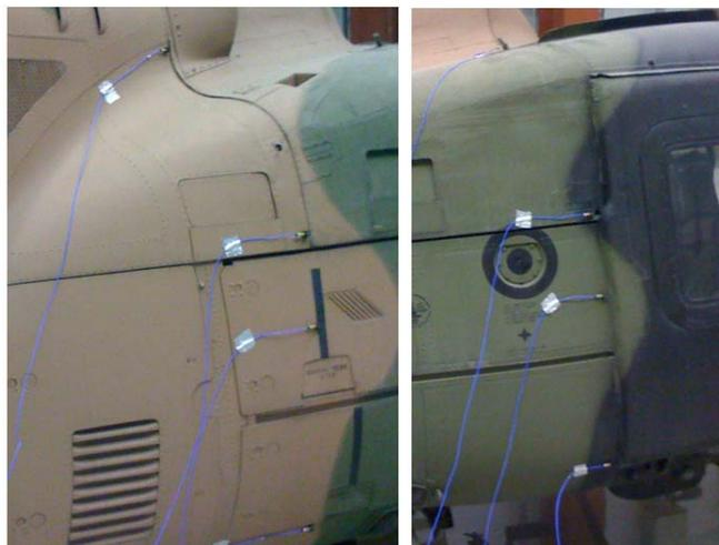
**Figure 5.9 Accelerometer locations at main body**
