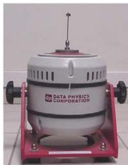
**Figure 3.4 Electro-dynamic shaker with stinger attachment**
