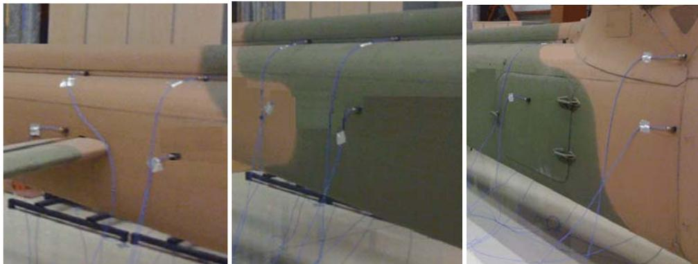
**Figure 5.8 Accelerometer locations at tail front**
