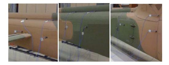
Figure 5.8 Accelerometer locations at tail front
