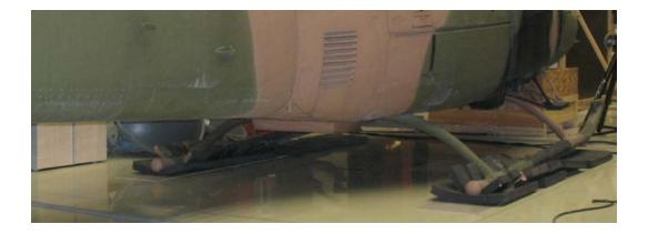
Figure 5.3 Foams that are used for free-free boundary condition.
