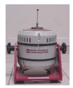
Figure 3.4 Electro-dynamic shaker with stinger attachment
