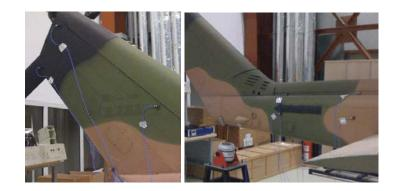
Figure 5.7 Accelerometer locations at tail end
