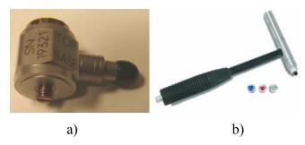
Figure 3.5 a) Force Transducer, b) Impact Hammer with different tips
