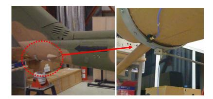
Figure 5.4 The part that connect stinger to the helicopter
