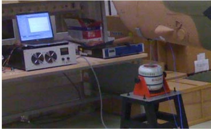
**Figure 5.11 Shaker, controller, and amplifier system**
