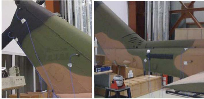
**Figure 5.7 Accelerometer locations at tail end**
