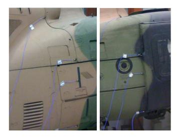
Figure 5.9 Accelerometer locations at main body
