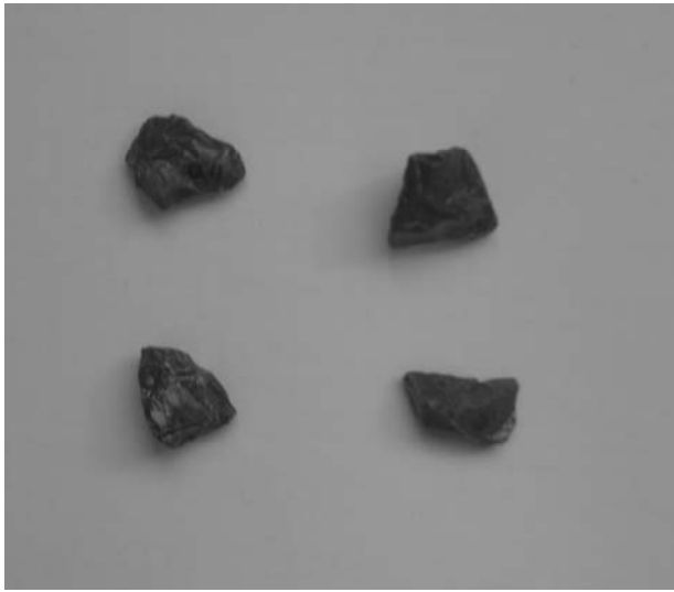
Figure III-5: Rough channel bed # R1 particles used in the experiments
