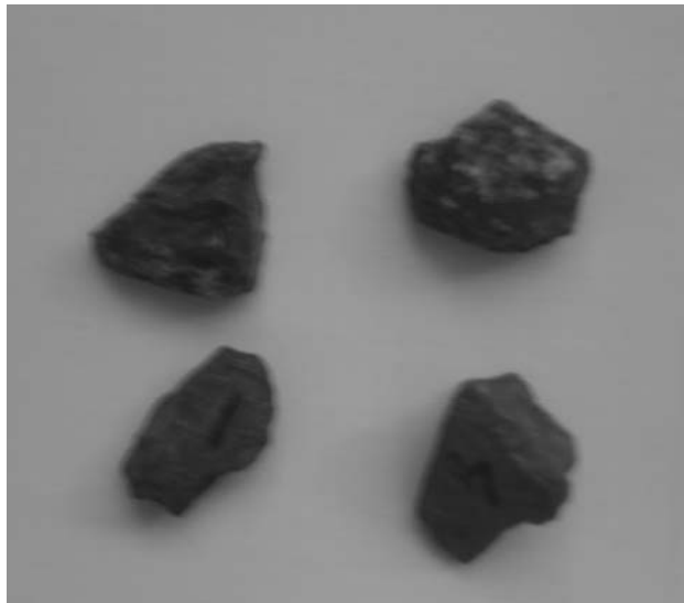
Figure III-6 Rough channel bed # R2 particles used in the experiments
