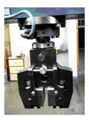
Figure 3.8: Tensile testing grip of the test machine
