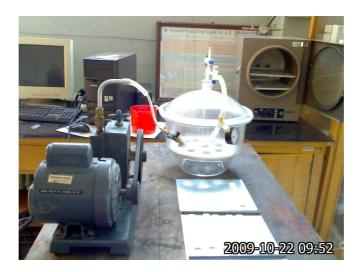
Figure 5.2: Dessicator - Vacuum Pump - Oven - Specimens on Plate
