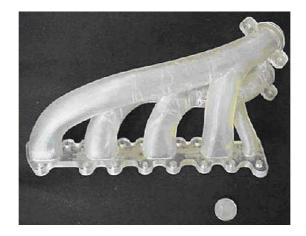
Figure 1.2: An engine manifold produced with SLA [10]
