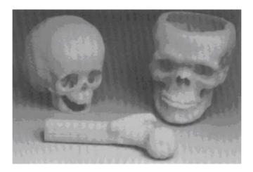
Figure 2.2: 2 human skulls with a femur produced via SLS [23]
