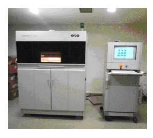
Figure 3.1: EOSINT P380 Laser sintering machine in Biltir, METU
