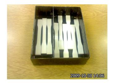
Figure 5.1: Specimens in container
