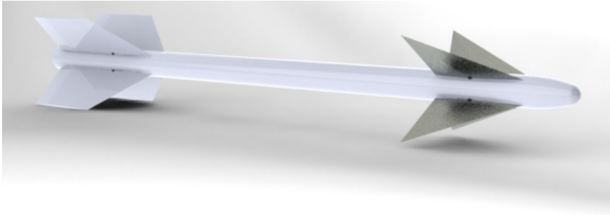
Figure 3.1 Baseline Configuration AIM 9D (Modeled in SolidWorks)
