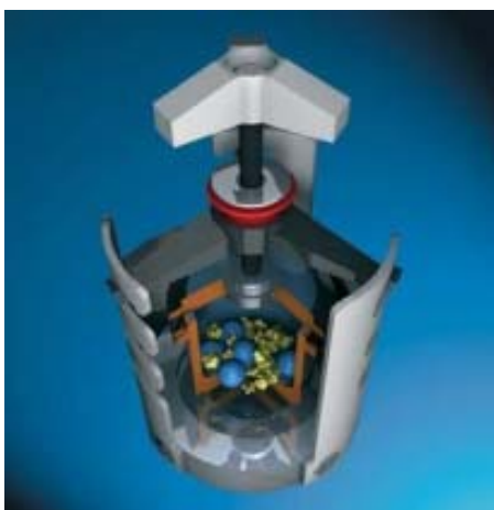
Figure 3.3 Representative sketch of the high energy ball mill used.
