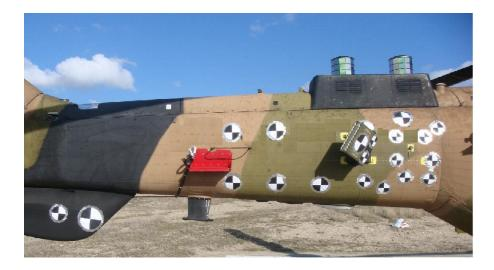
Figure 15-Target Positions on Helicopter Fuselage (Tail Boom)
