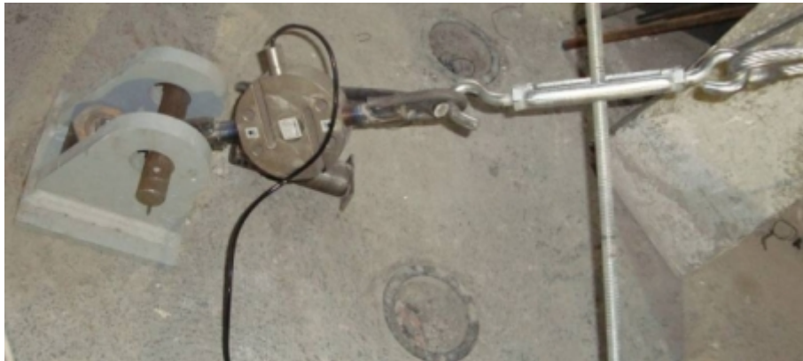
Figure 2.13: Load cell and turnbuckle with base plate
