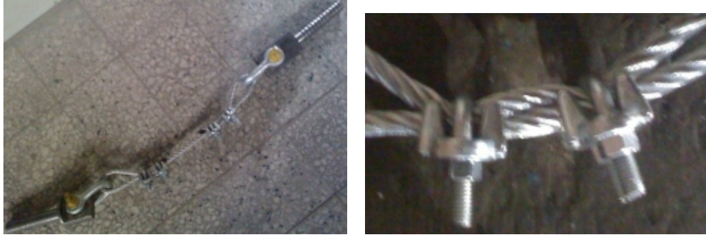
Figure 2.12: Third specimen before test and its end locks
