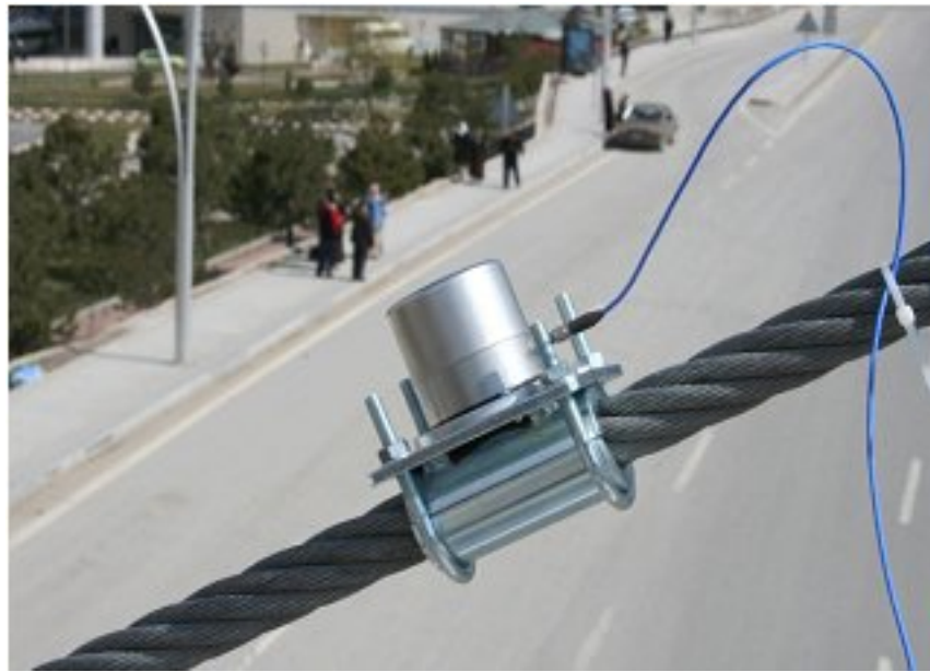
Figure 2.1: Accelerometer Attached to Cable (in Field Study)
