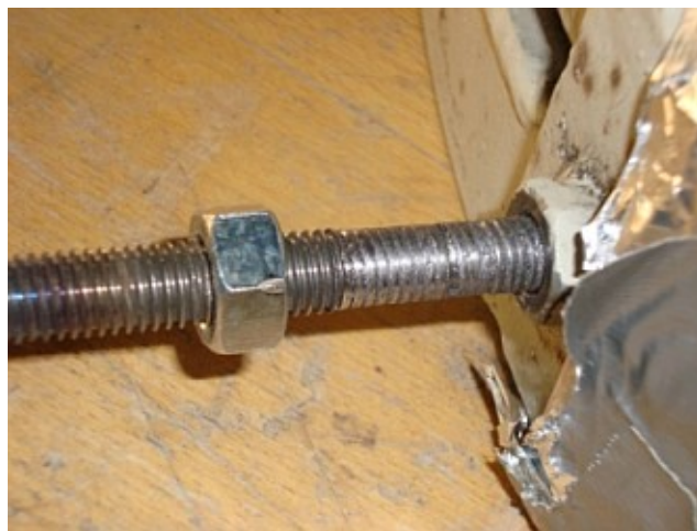
Figure 2.15: Distorted central screw
