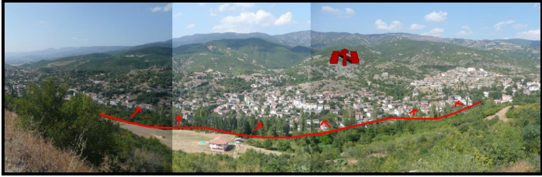
Figure 3.8. Main scarps of landslides from the landslide crown. The photograph is taken from the point having coordinates of UTM Zone 37T, 4494901N and 327557E.
