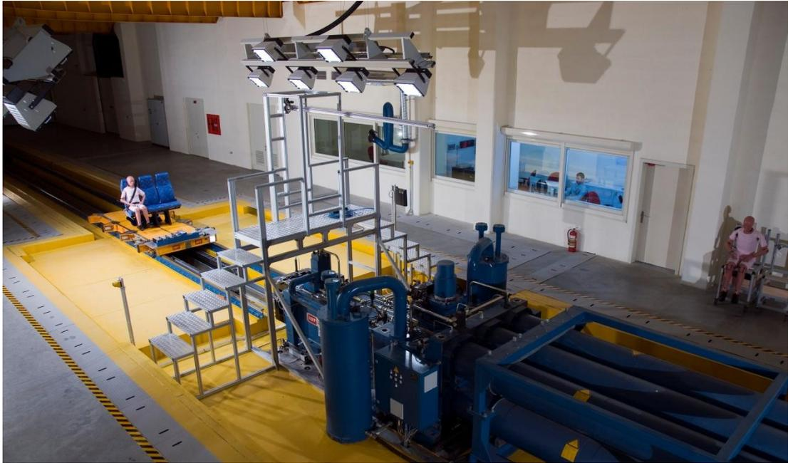
**Figure 1.1 Crash Test System at METU-BILTIR Center**
