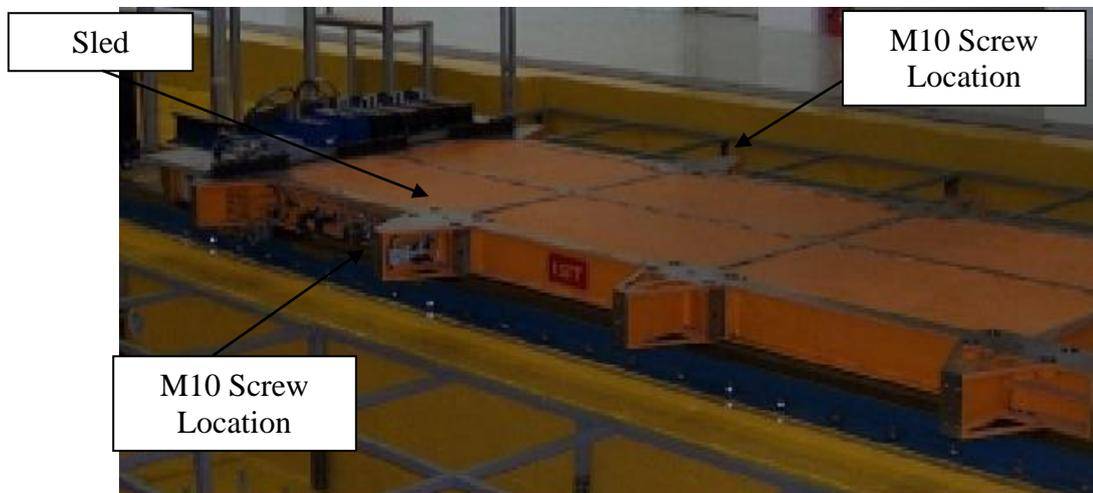
**Figure 2.4 Sled of the Crash Test System**
