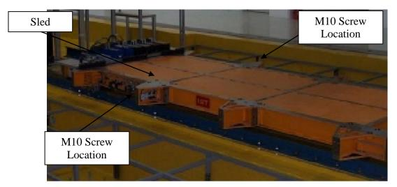
Figure 2.4 Sled of the Crash Test System
