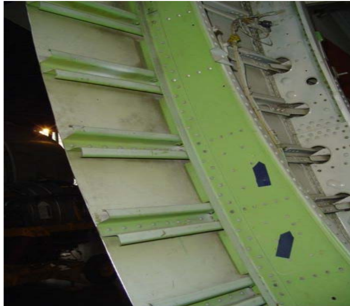
Figure 1.2: Typical Example of a Developed Semi-monocoque Structure
