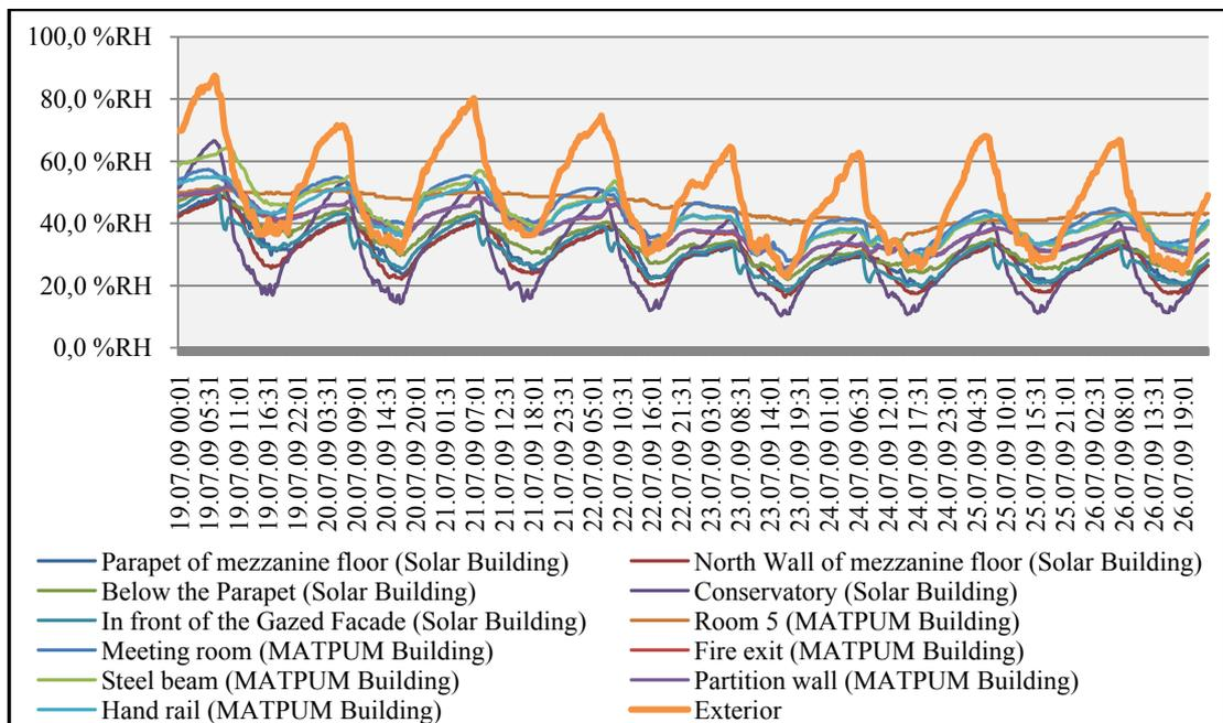
**Figure 4.6** Humidity chart of the MATPUM Building & Solar Building (19-26 July 2009)
