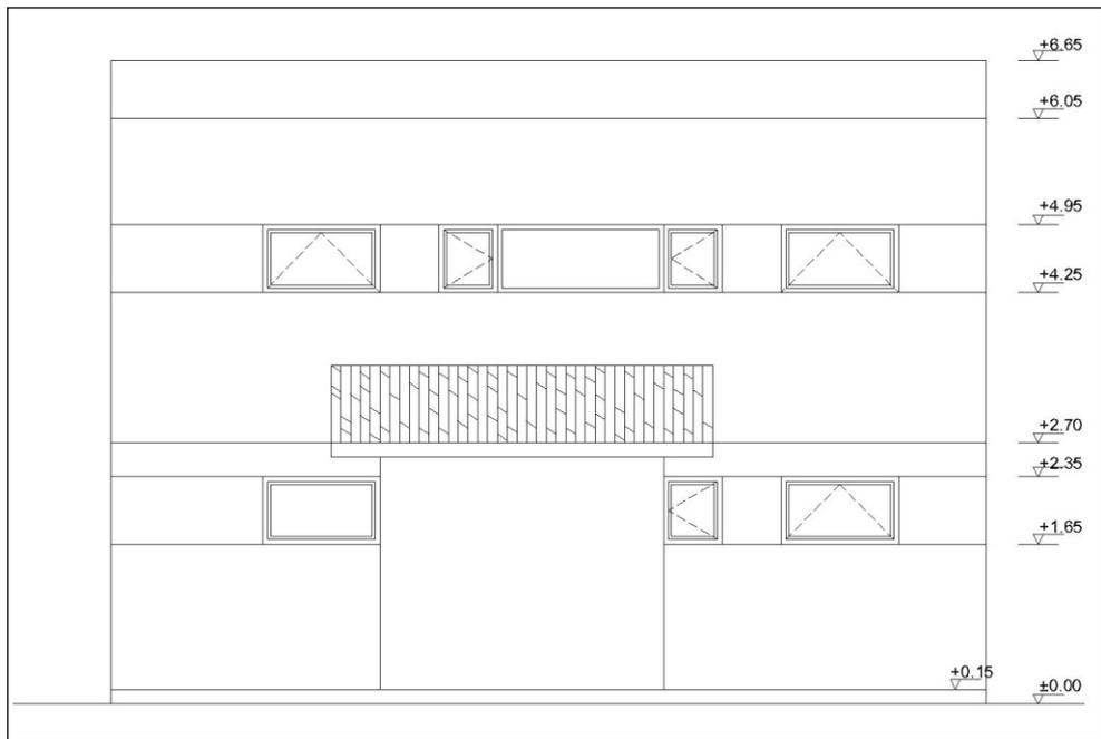
**Figure B.5** North Elevation of Solar Building
