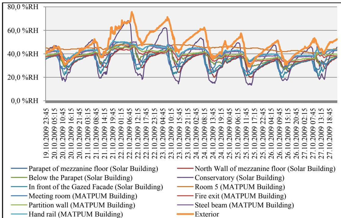
**Figure 4.10** Humidity chart of the MATPUM Building & Solar Building (20-27 July 2009)
