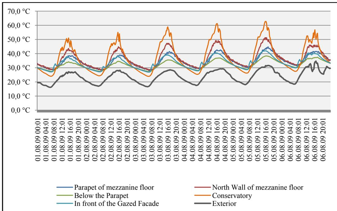
**Figure C.15** Temperature chart of the Solar Building (01-06 August 2009)
