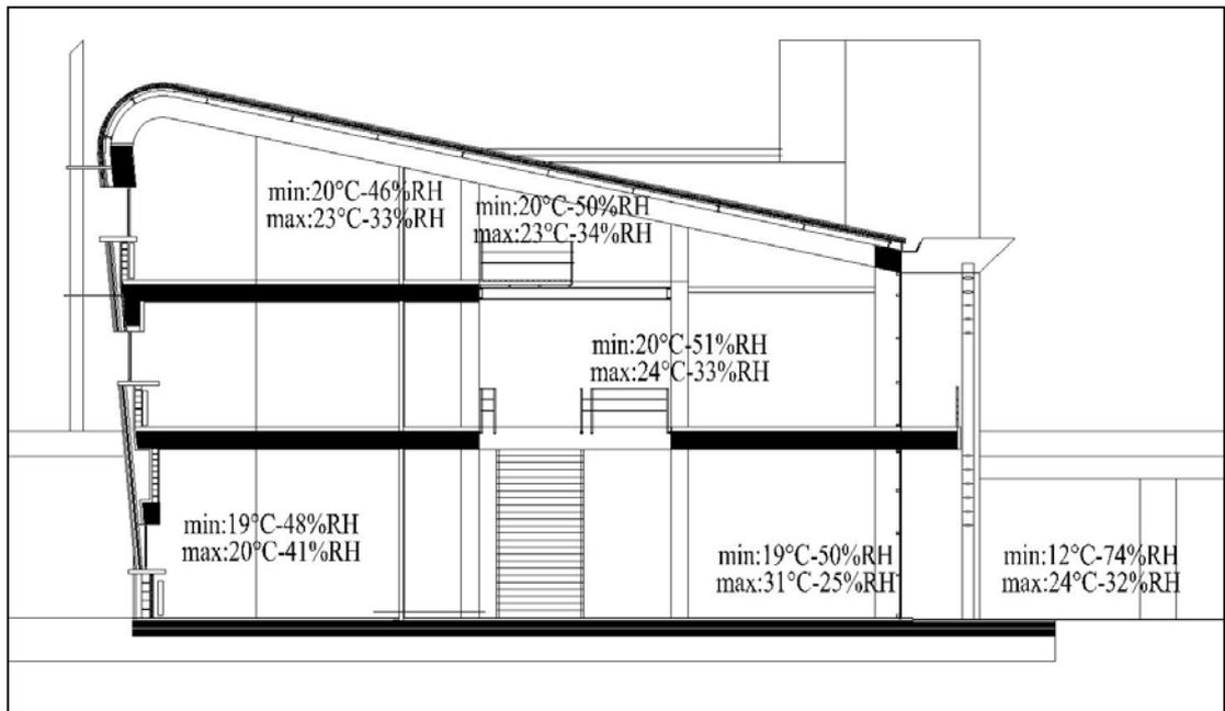
**Figure 4.11** Section showing the minimum and maximum temperature and humidity values at different locations of the MATPUM Building (20-27 October 2009)
