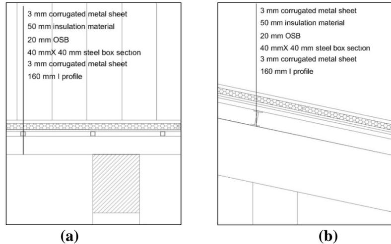
**Figure 3.1** System detail from the roof of the MATPUM Building
