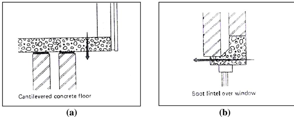
**Figure 2.4** Thermal bridges **a.** At cantilevered concrete floor **b.** At boot lintel over window (Source; McMullan, 1998, p. 46)
