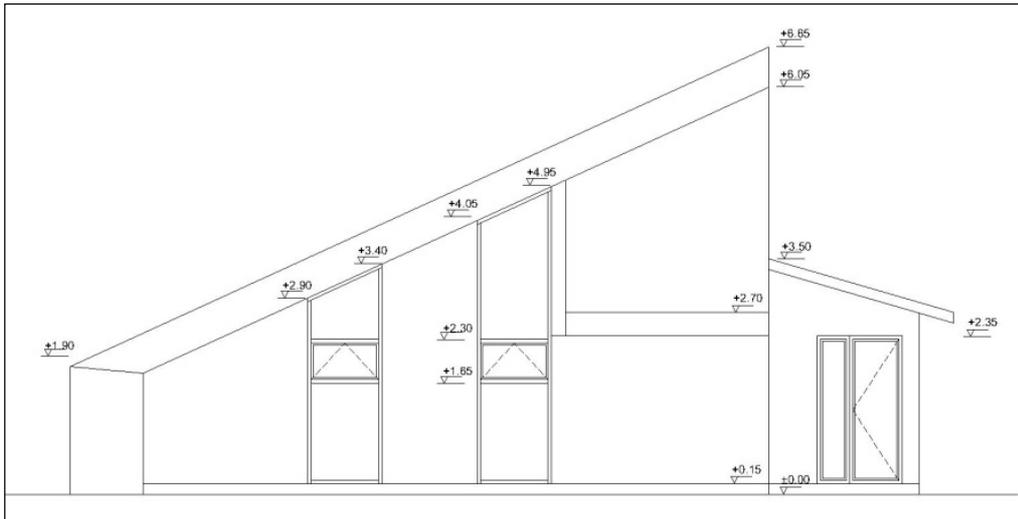
**Figure B.4** East Elevation of Solar Building
