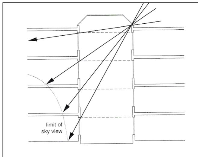
**Figure 2.11** The effects of atrium height (Source; Baker & Steemers, 2000, p. 69)
