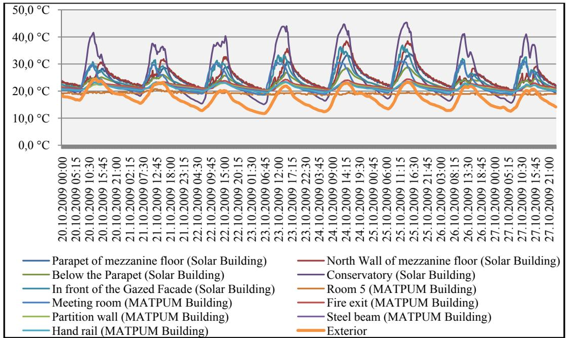
**Figure 4.9** Temperature chart of the MATPUM Building & Solar Building (20-27 July 2009)
