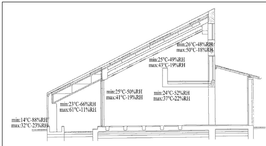
**Figure 4.8** Section showing the maximum and minimum temperature and humidity values at different locations of the Solar Building (19-26 July 2009)
