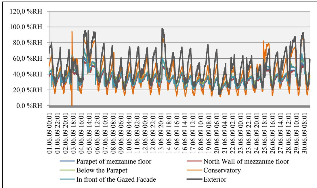
**Figure C.12** Humidity chart of the Solar Building (01-30 June 2009)
