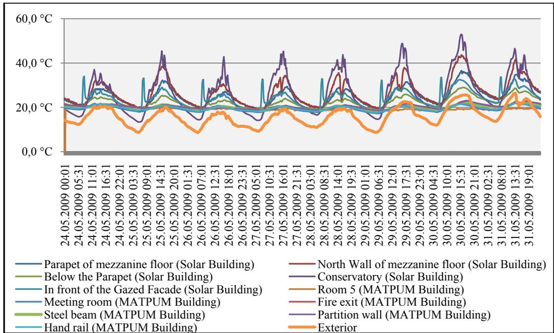
**Figure 4.1** Temperature chart of the MATPUM Building and the Solar Building (24-31 May 2009)
