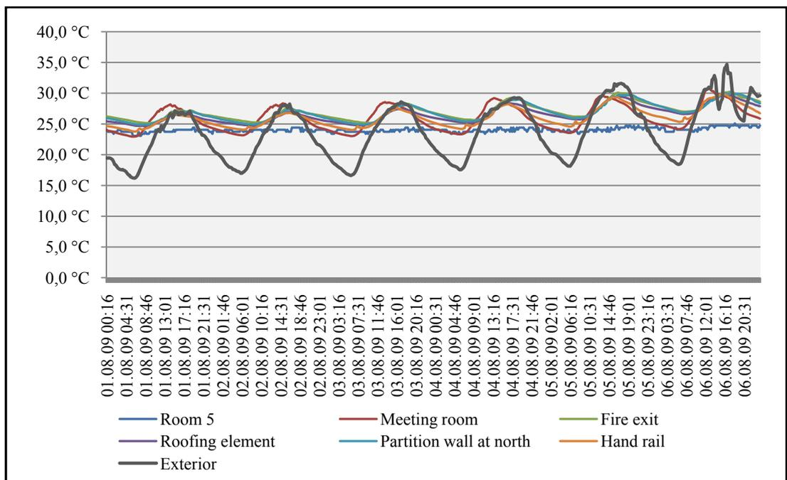
**Figure C.5** Temperature chart of the MATPUM Building (01-08 August 2009)
