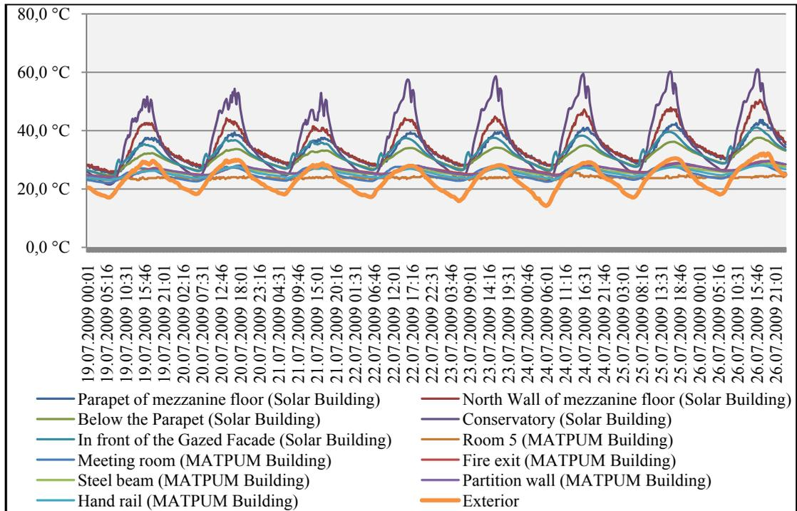
**Figure 4.5** Temperature chart of the MATPUM Building & Solar Building (19-26 July 2009)
