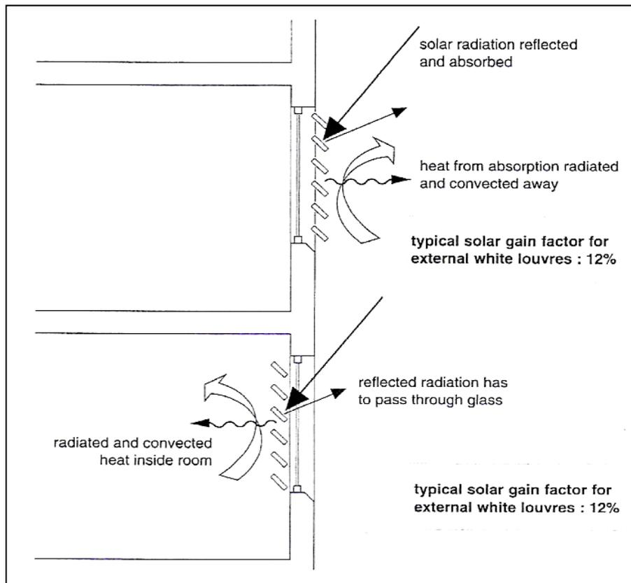
**Figure 2.6** The performance of internal and external louvers (Source; Baker & Steemers, 2000, p. 32)
