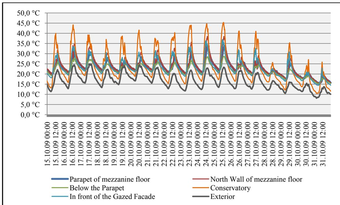
Figure C.17 Temperature chart of the Solar Building (15-31 October 2009)
