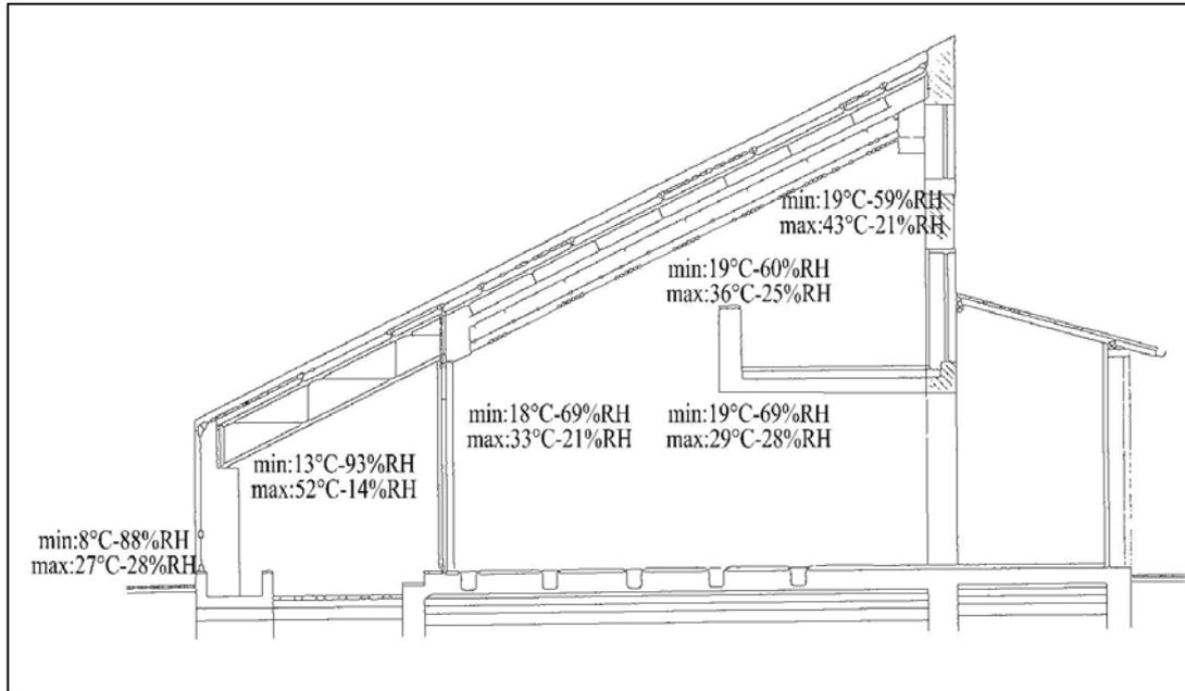
**Figure 4.4** Section showing the minimum and maximum temperature and humidity values at different locations of the Solar Building (24-31 May 2009)
