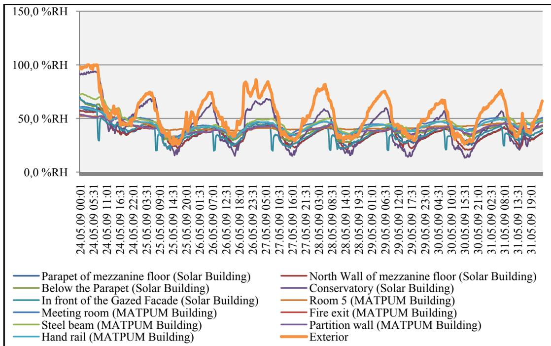
**Figure 4.2** Humidity chart of the MATPUM Building and the Solar Building (24-31 May 2009)
