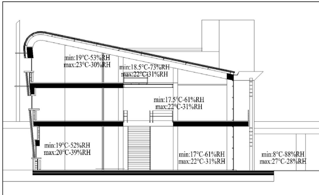
**Figure 4.3** Section showing the minimum and maximum temperature and humidity values at different locations of the MATPUM Building (24-31 May 2009)
