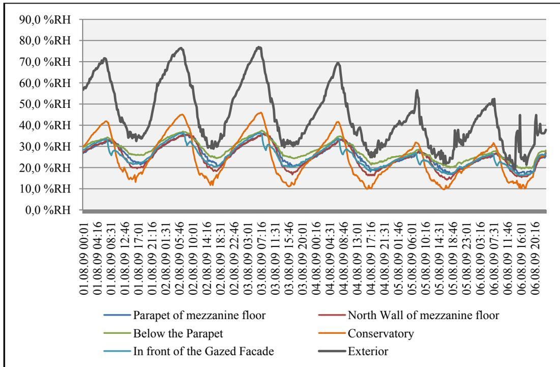
Figure C.16 Humidity chart of the Solar Building (01-06 August 2009)
