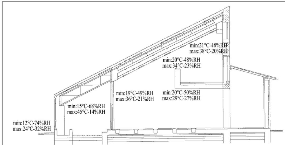
**Figure 4.12** Section showing the maximum and minimum temperature and humidity values at different locations of the Solar Building (20-27 October 2009)
