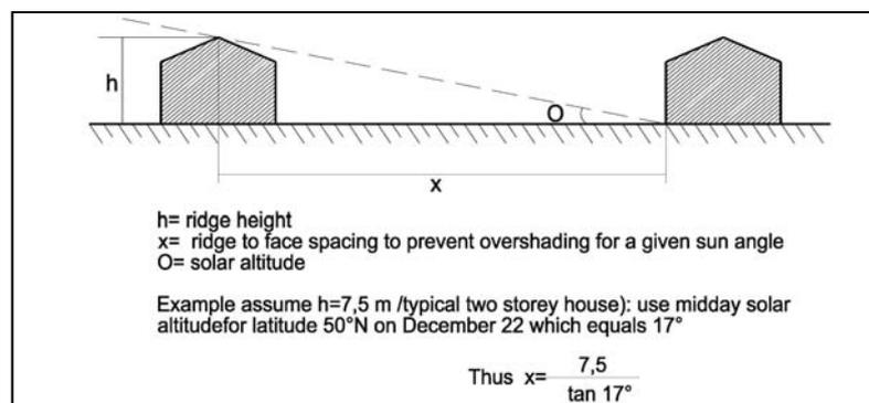
**Figure 2.1** Calculations for minimum over shading
