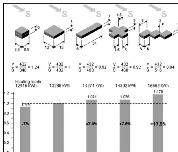
**Figure 2.3** Different surface to volume ratios according to different forms (Source; Gratia & De Herde, 2002, p.478)
