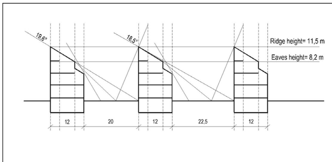
**Figure 2.2** South facing rows with optimized distances for solar incidence on building and open areas (Source: Gonzalo & Haberman, 2006, p.35)
