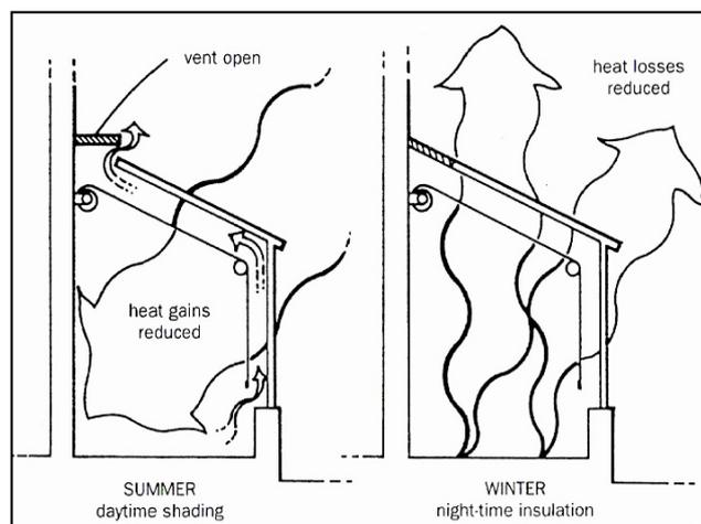
**Figure 2.8** A movable shading device used in conservatory
