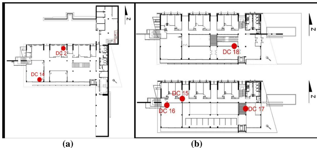
**Figure 3.7** The locations of the data loggers on the plans of the MATPUM Building
