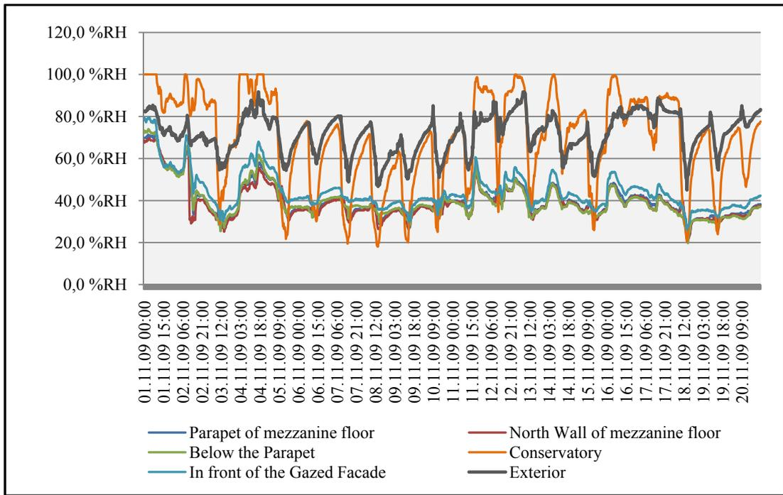
**Figure C.20** Humidity chart of the Solar Building (01-20 November 2009)
