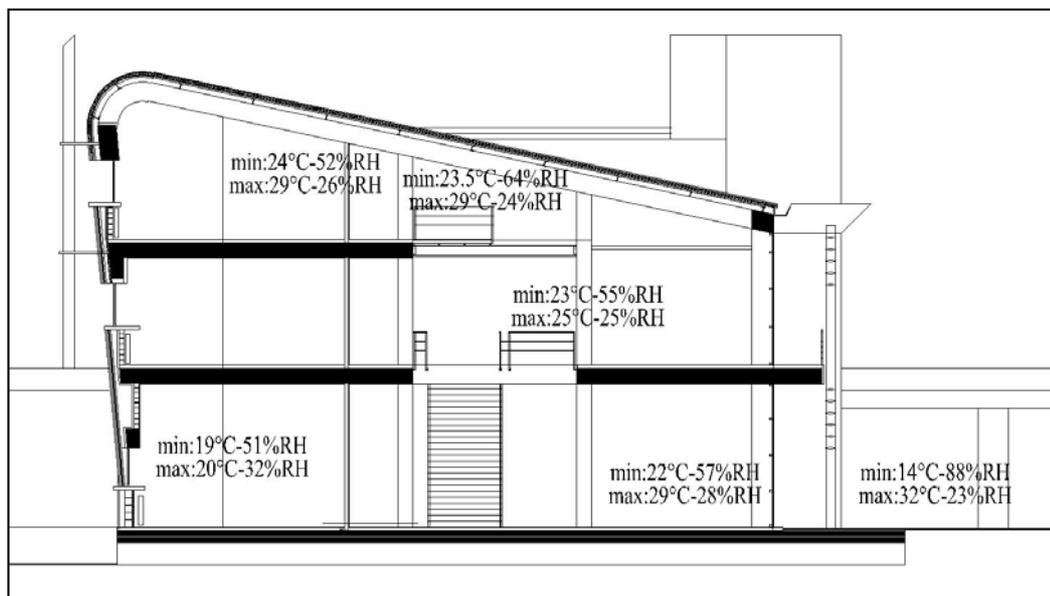
**Figure 4.7** Section showing the maximum and minimum temperature and humidity values at different locations of the MATPUM Building (19-26 July 2009)
