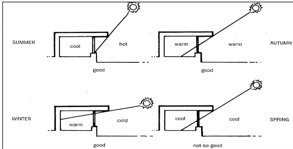
**Figure 2.5** The effects of roof overhang on solar radiation in different seasons (Source; Waterfield, 2006, p. 26)
