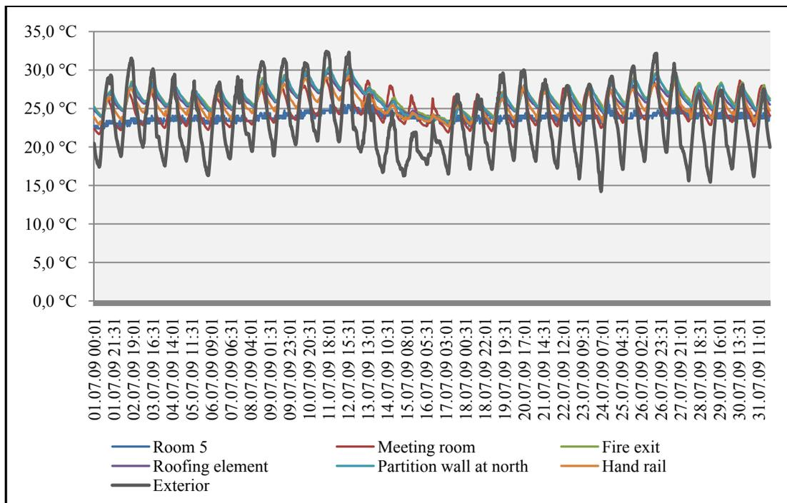
**Figure C.3** Temperature chart of the MATPUM Building (01-31 July 2009)
