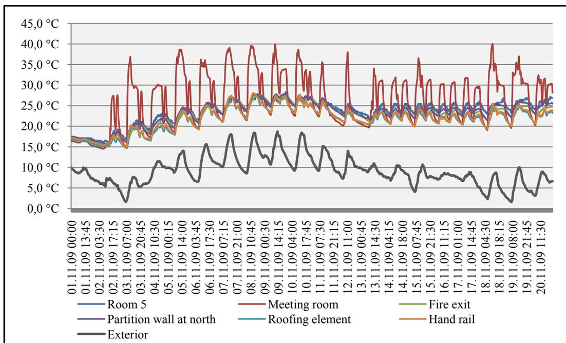
**Figure C.9** Temperature chart of the MATPUM Building (01-20 November 2009)
