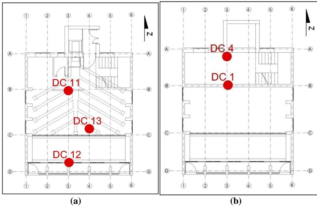
**Figure 3.11** Locations of data loggers shown on floor plans of the Solar Building
