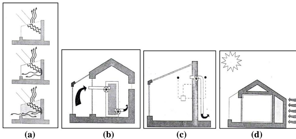
**Figure 2.7** Passive heating strategy of a sunspace **a.** Solar collection **b.** Heat storage **c.** Heat distribution **d.** Heat conservation
