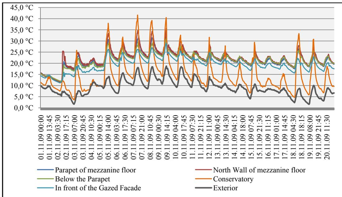
**Figure C.19** Temperature chart of the Solar Building (01-20 November 2009)
