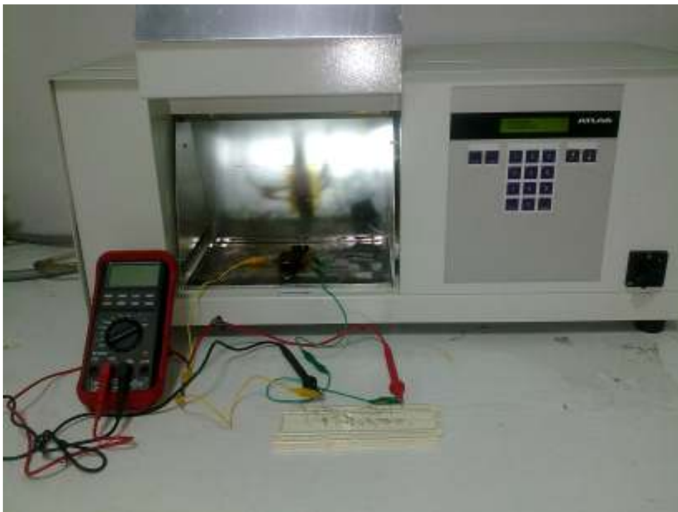
Figure C.1. Current-voltage measurement setup.
