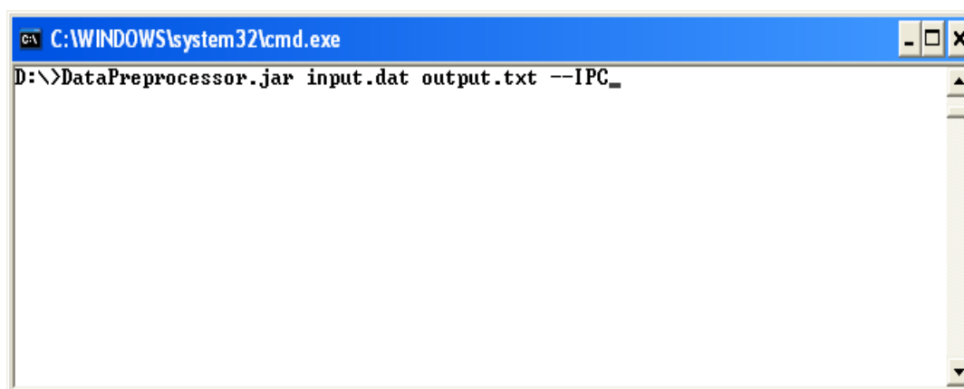
Figure 62: Running pre-processor from command line
