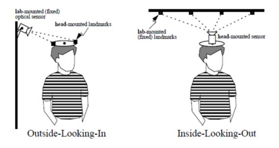
Figure 2.2: Outside-in and Inside-out Tracking [23]. (Courtesy of Greg Welch)
