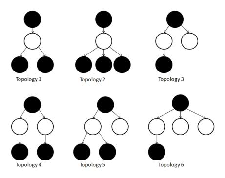
Figure 3.8: Topology trees when tree depth is 2 and maximum number of leaves is 3.
