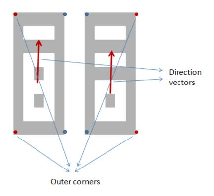
Figure 3.13: 2D direction vectors and four outer corners that are used for obtaining the transformation matrix.
