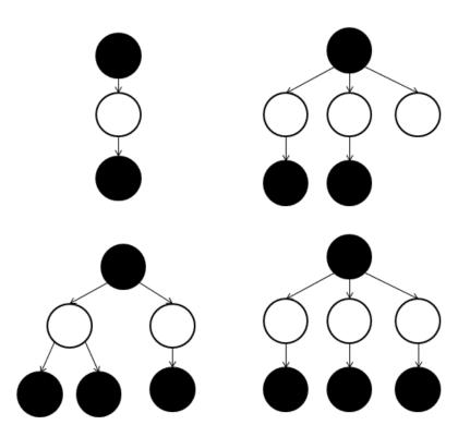
Figure 3.9: First topology is eliminated since it is not complex enough. Other topologies are eliminated since they require more than 9 pixels in height.
