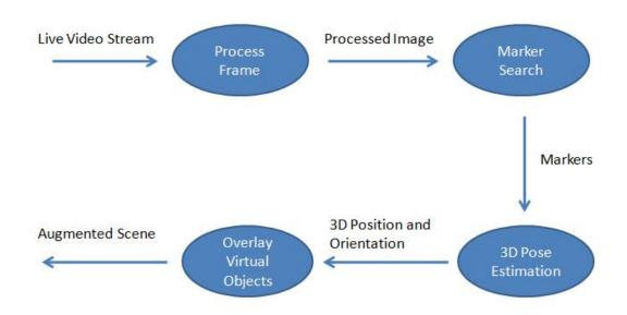
Figure 2.4: Overall Structure of Marker Based Vision Systems.
