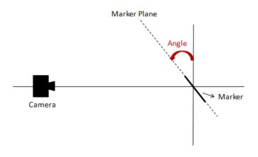
Figure 4.2: Camera-marker angle
