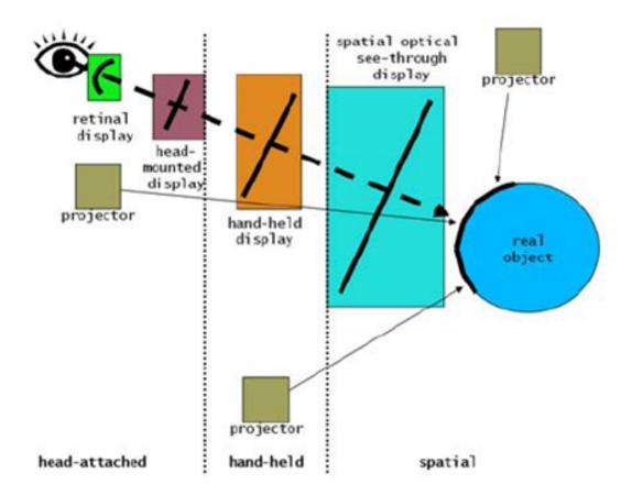
Figure 2.3: Categorization of Display Technologies [8]. (Courtesy of Oliver Bimber)
