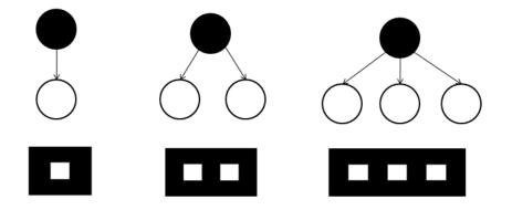
Figure 3.6: Three possible topology trees for tree depth of 1 are shown above. For each topology tree, corresponding geometry is shown below.
