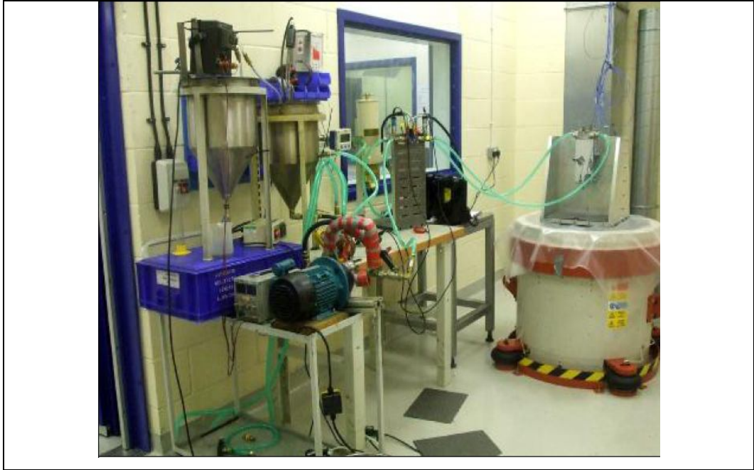
Figure 5.7 ISO 13353 Test Stand with vibration rig modification
