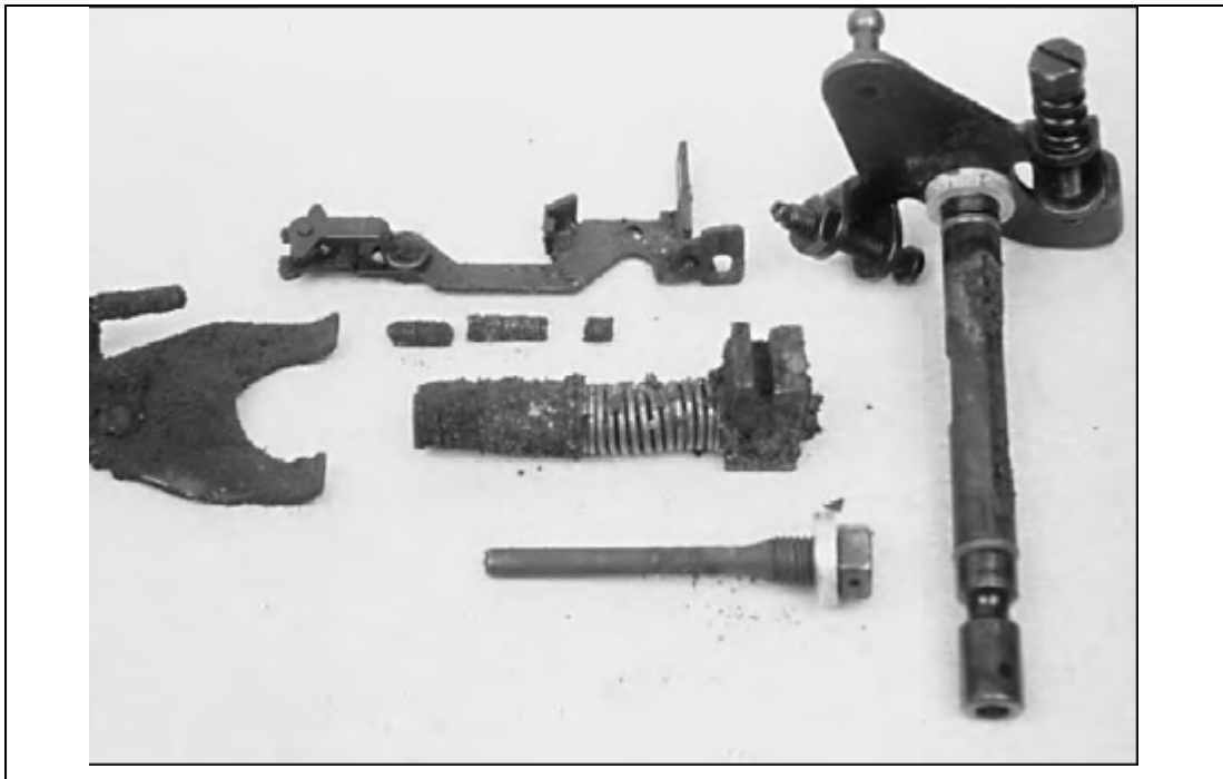
Figure.2.16 . Fuel Metering and Governing Components of A Distributor Type Injection Pump Destroyed By Rusty Water Contamination
