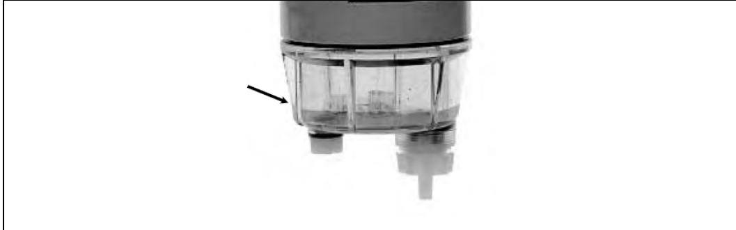
Figure. 2.42 Water is easily visible in the collection bowl.
