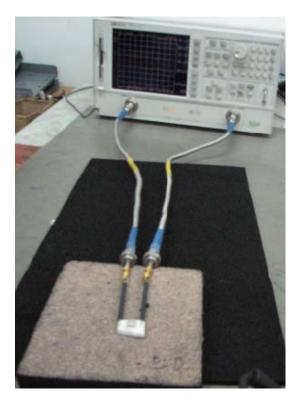
Figure 4-15: A simple experimental set-up used to measure transmission spectrum of SRR structures in air.
