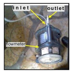
Figure 5.3 Inlet and outlet of the flowmeter.
