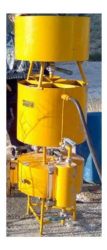
Figure 5.15 Steam Separator used in the Kızıldere geothermal field.
