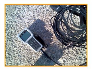
Figure 5.11 The Multiparameter measurement device used in the geothermal fields.
