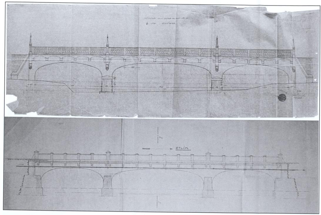
**Figure 4.36** Up: Façade proposal for the Etlik Bridge with minaret-like newels. Down: Longitudinal section drawing of the Etlik Bridge, 1936. Source: Unclassified documents from the State National Archives-Republican Archives, KGM Fund, Binder no: 1839
