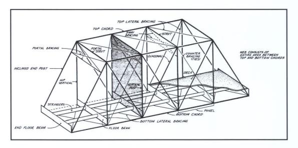
Figure B.6 Structural elements in a truss. Source: Historic American Engineering Record, The Society for Industrial Archeology, Record No. HAER TI-1
