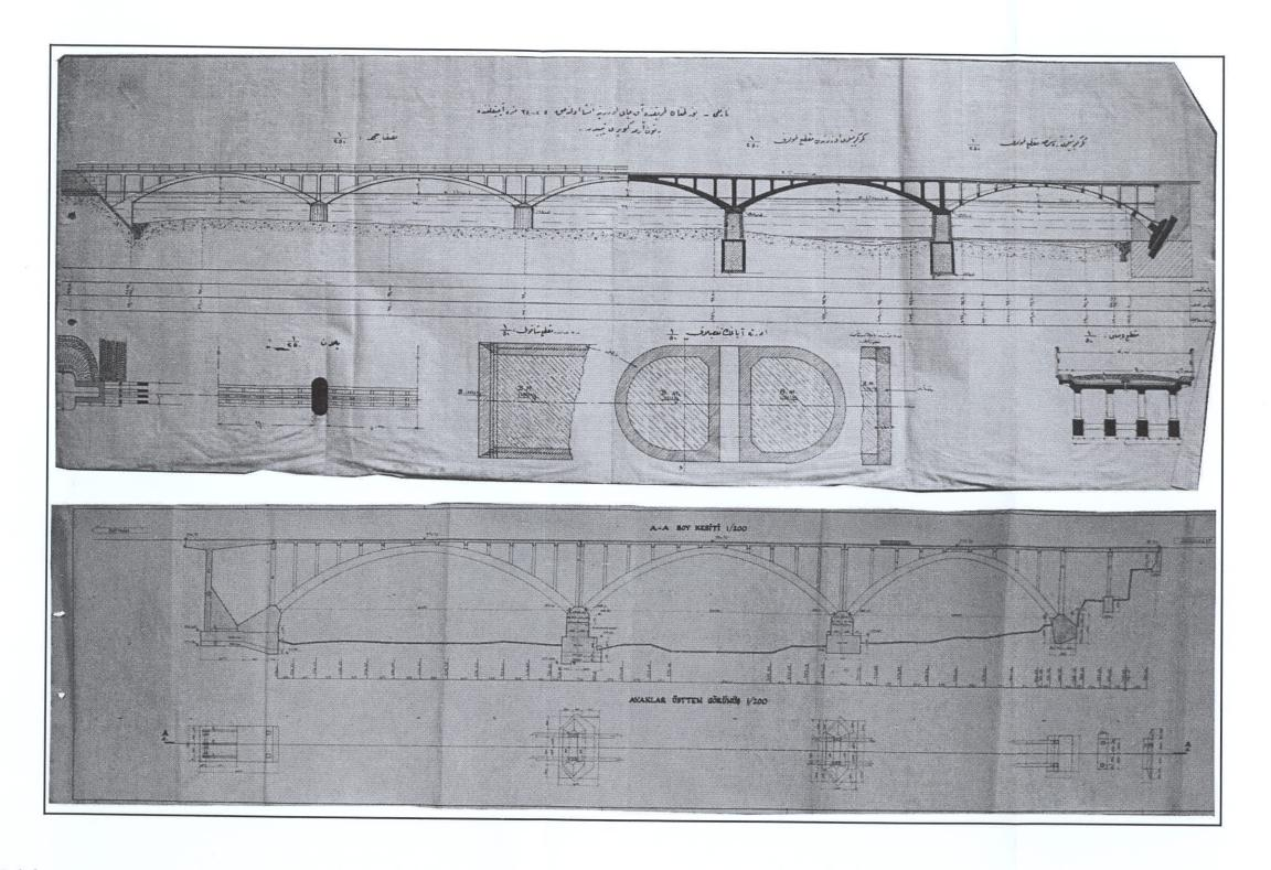
**Figure H.10** Reinforced concrete bridge technology had remained almost the same until 1960. Drawings of two reinforced concrete arch bridges Akçay Bridge in 1928 (above) and Hasankeyf Bridge in 1956 (below). Source: Unclassified documents from the State National Archives-Republican Archives, KGM Fund, Binder no: 9616-1 and 9616-2
