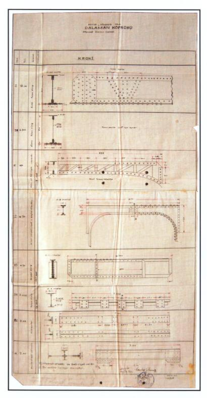
**Figure 4.11** List of the steel elements remained. From the inventory list produced in 1930s for construction of 70 m span steel town lattice truss type Dalaman Bridge. Source: Unclassified document from the State National Archives-Republican Archives, KGM Fund, Binder no. 2203
