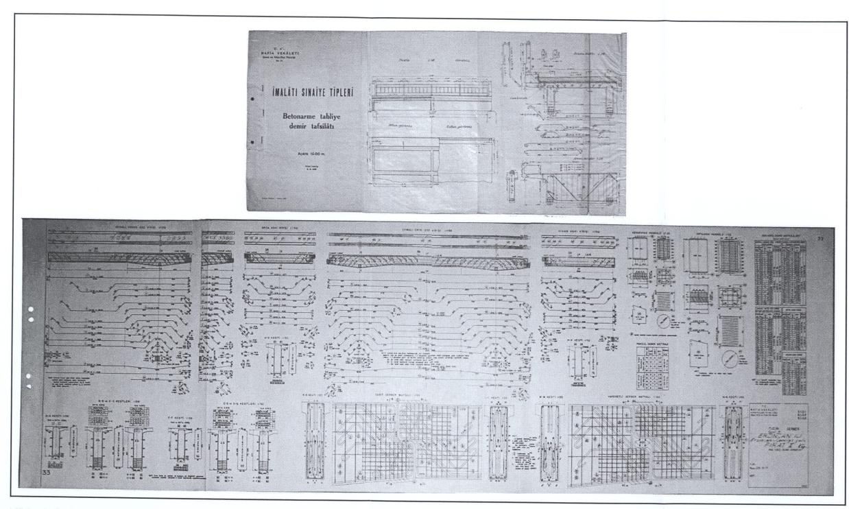
**Figure 4.28** Standardization of road bridges in 1950s. Ready-to-built gerber bridge plans which were for 10 meters (above) increased to for 25 meters (below), produced by the Ministry of Public Works, applied in Fırat II bridges in 1957. Source: Unclassified documents from the State National Archives-Republican Archives, KGM Fund, Binder no: 8113
