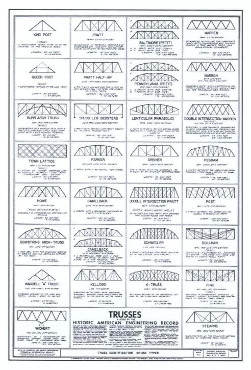
Figure B.5 Graphic showing various truss types. Source: Historic American Engineering Record, The Society for Industrial Archeology, Record No. HAER TI-1
