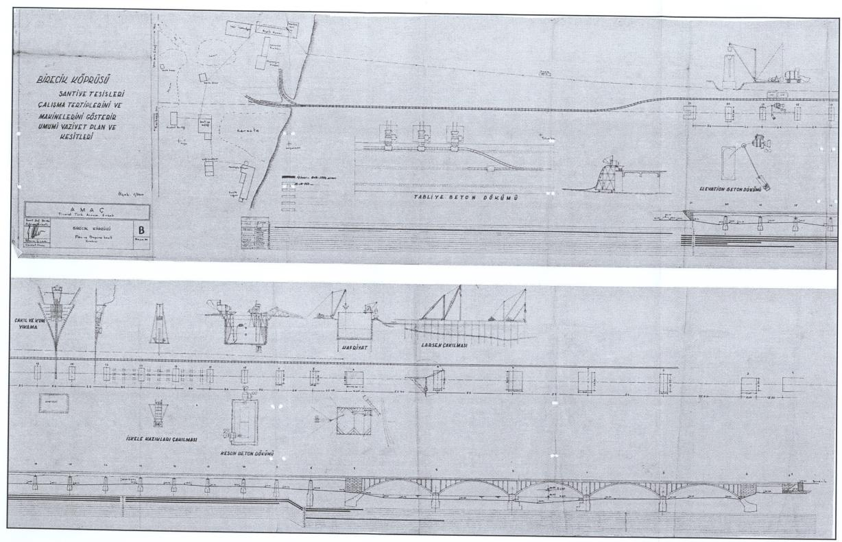
Figure 4.49 Site plan of Birecik Bridge showing the equipments in the site. Source: KGM Archives
