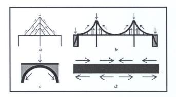
**Figure B.1** (a) Tension (cable-stayed), (b) tension (suspension), (c) compression (arch), and (d) tension/compression. Source: Wilson, T., Wash Bridge Competition: Bridge Engineering. (Available at http://www.phlf.org/downloads/education/Edu\_WabashBridgeDesign.pdf on 2.2.2008)
