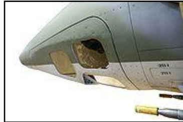
Figure 1.2: Camera bay of a reconnaissance Mirage III R
