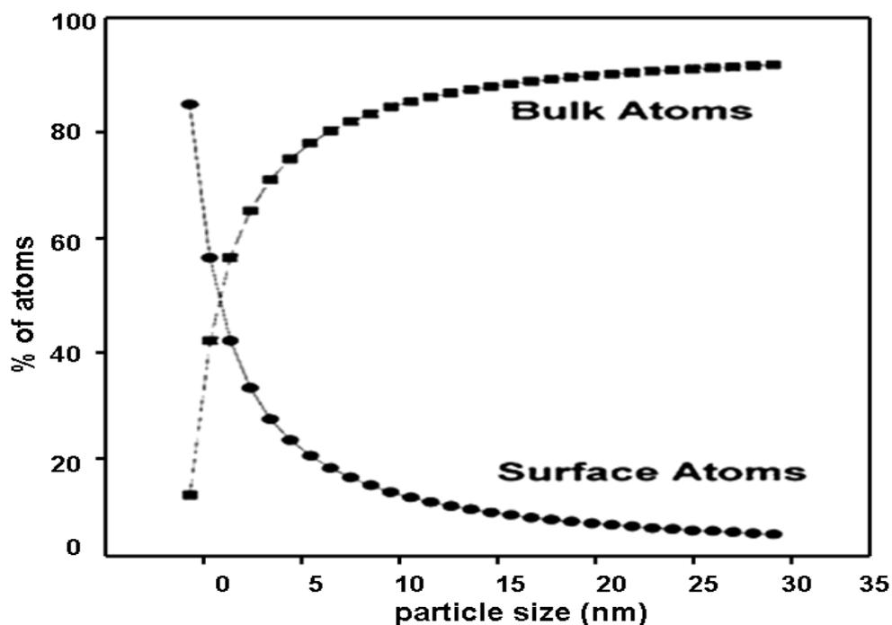
**Figure 2.3.** Calculated surface to bulk ratios for solid metal particles versus size (adopted from the literature [31])
