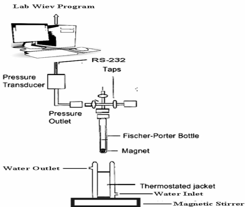
**Figure 3.1.** The experimental setup used in performing the catalytic methanolysis of ammonia borane and measuring the hydrogen generation rate.
