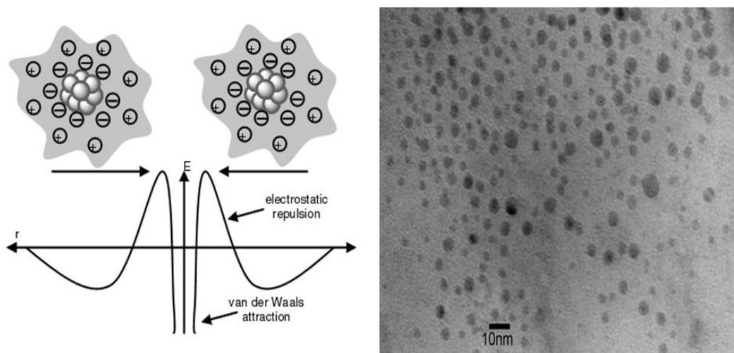
**Figure 2.4.** (a) Schematic representation of electrostatic stabilization, (b) Acetate stabilized Ru(0) nanoclusters (adopted from literature [61]).
