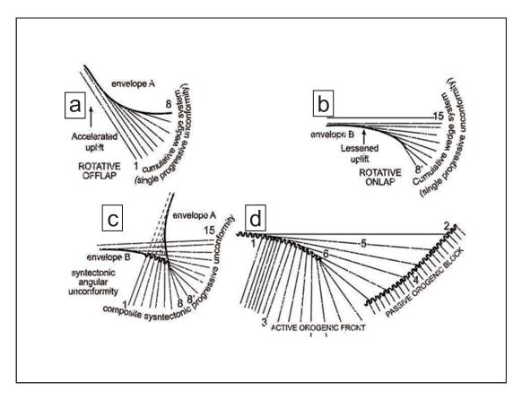
Figure 11. Conceptual configuration of progressive unconformities in area where tectonic activity and sedimentation are coupled. The numbers 1-15 are time lines (adopted from Riba 1976).
