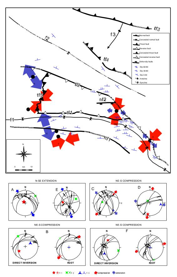
Figure 15. a) Major structures and paleostress orientations. b) Cylographic traces, slickensides and constructed paleostress configurations. Note that R2DT method yielded more reliable results than Direct Inversion methods of Angelier (1988).
