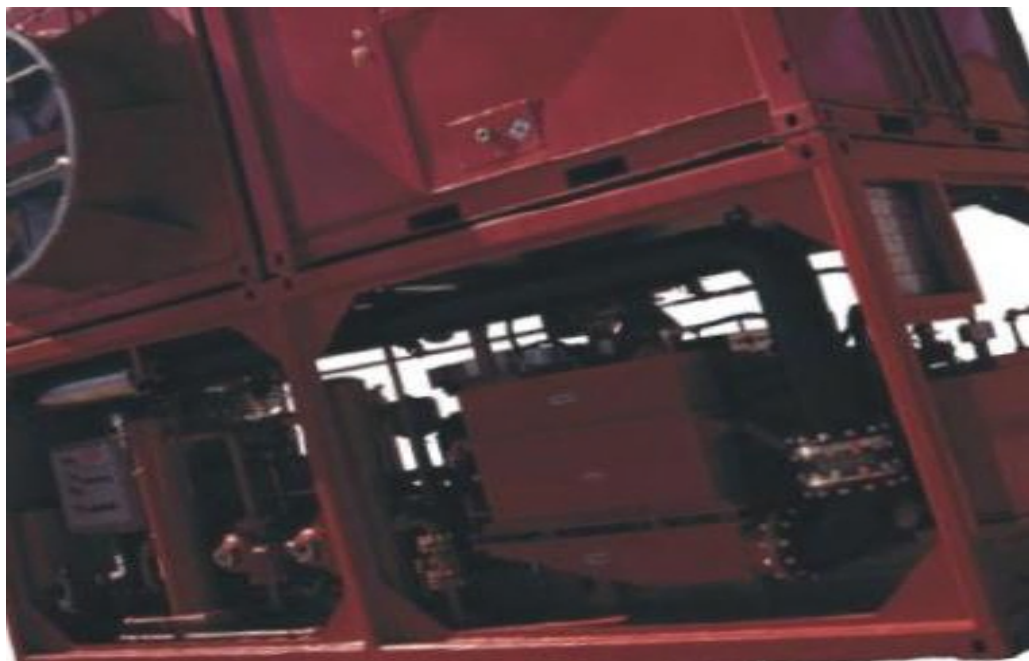
Figure 66 Nitrogen Generation/Production Unit (NGU/NPU) 59
