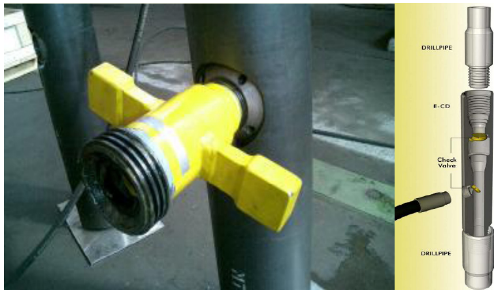
Figure 73 Continuous Circulation Valve (CCV) 24
