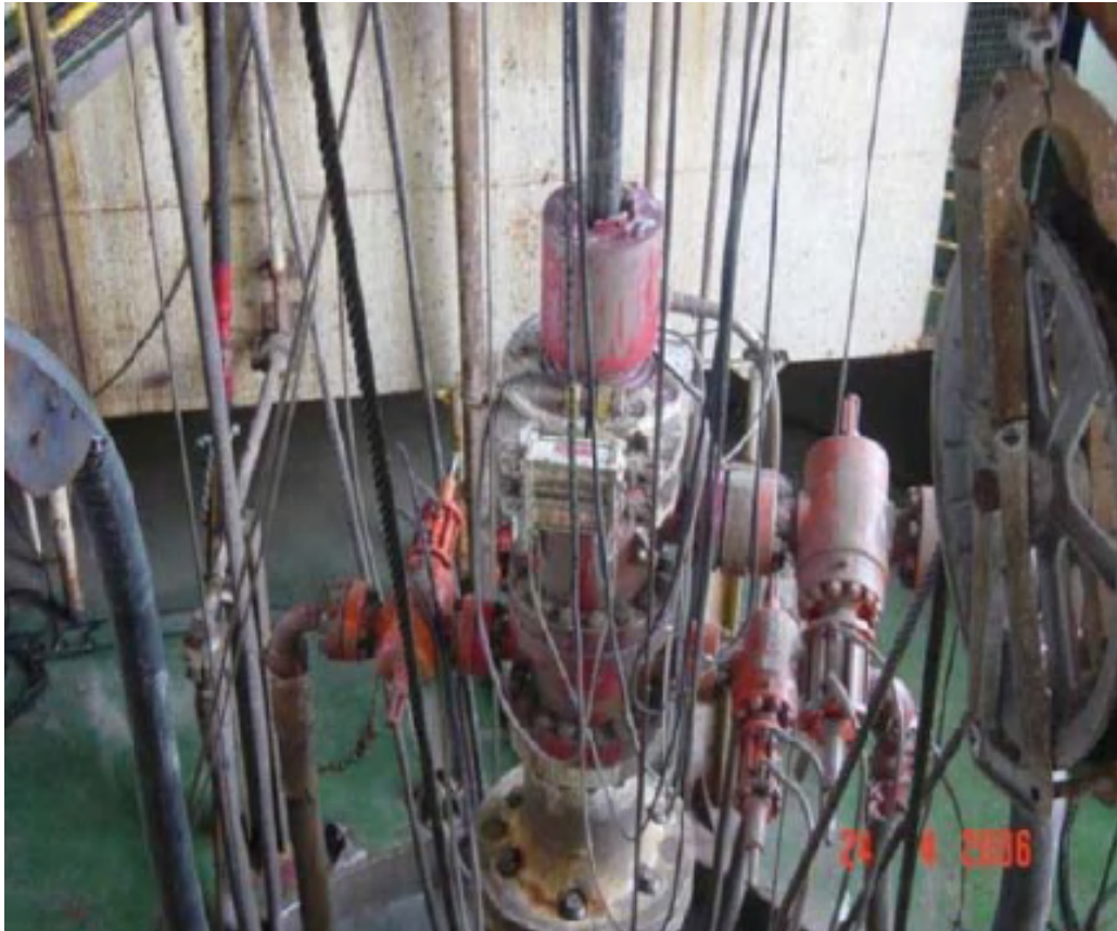
Figure 48 Subsea RCD (SSRCD) installation in moon pool 36
