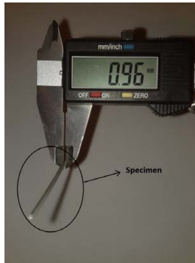
Figure 3.10: Electrical resistivity specimen obtained by wire-erosion technique
