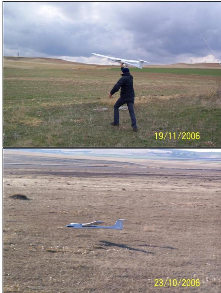
Figure 2 Hand launch (top) and belly landing of “Güventürk”
