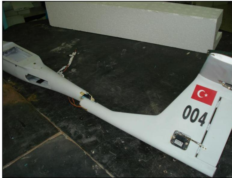
Figure 55: Crush damage on the tail of the UAV
