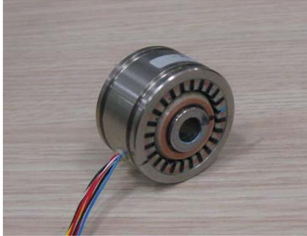
Figure A-4 5 kHz resolver used in experimental set-up
