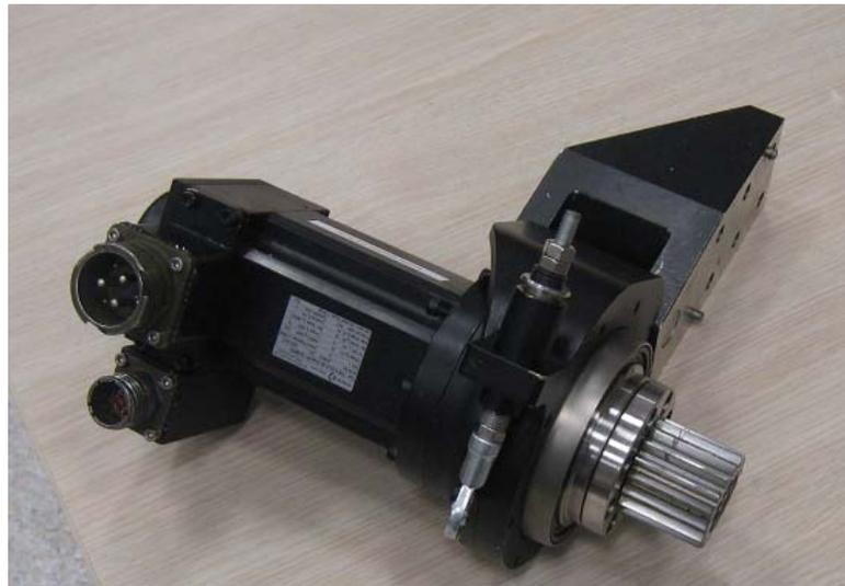
Figure A-5 AC servo motor used in the experimental set-up
