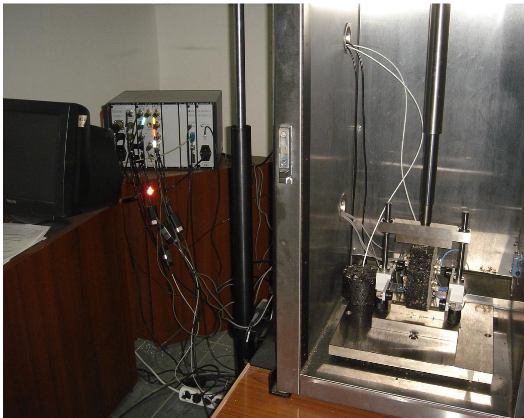
Figure 3.10 Universal testing machine (UTM-100) used for the resilient modulus tests
