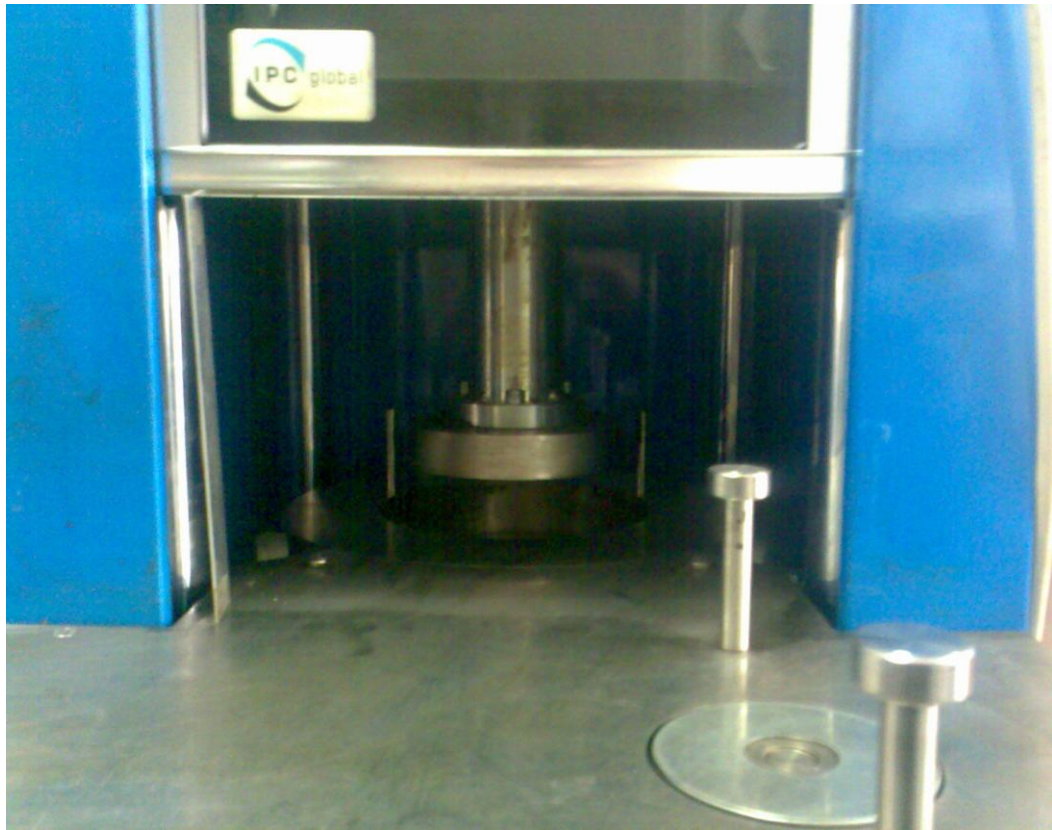
Figure 3.6 the place of the mold in the gyratory compactor
