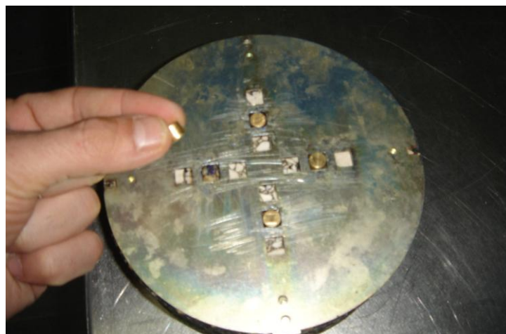
Figure 3.11 Gluing of LVDT installation fixtures onto the test specimen by the help of a mould
