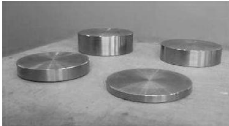
Figure 4.4 Inserts of the Die Set after Machining Operations
