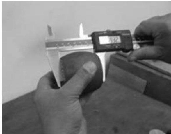
Figure 4.17 Measuring the Final Height of a Specimen
