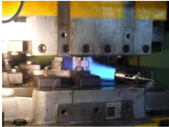
Figure 4.13 Preheating of the Forging Dies
