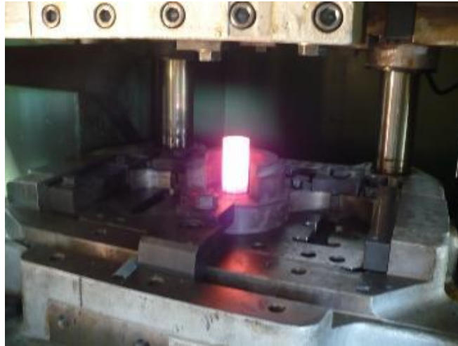
Figure 4.15 A Specimen Waiting to be Forged Between the Dies
