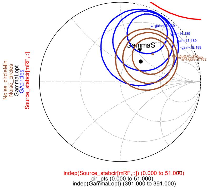
Figure 4-20: Gain, Stability and Noise Circles of FHX13X on Smith Chart
