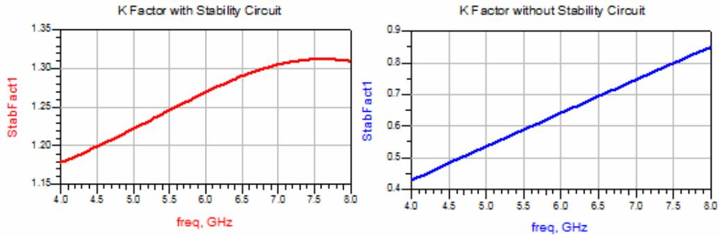
Figure 4-6: Stability Factor-K with and without Stability Circuit
