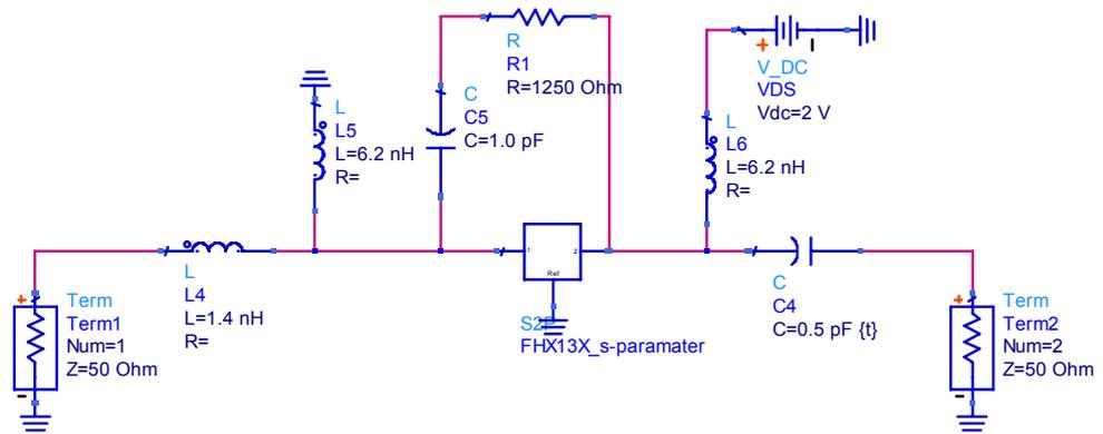
Figure 4-22: Final Schematic of FHX13X LNA Circuit
