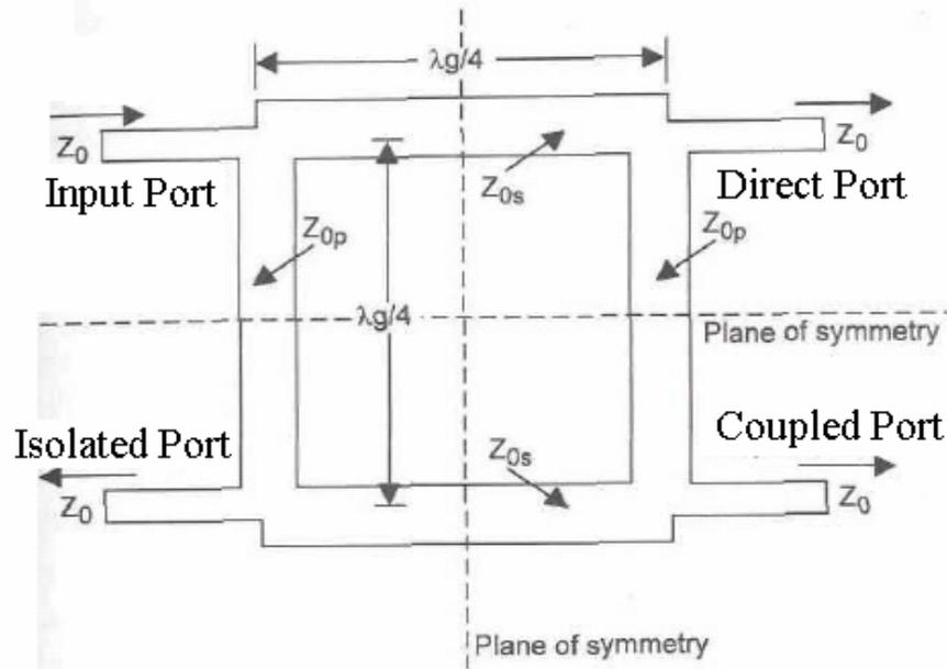
Figure 3-3: Layout of a Branch-Line Coupler
