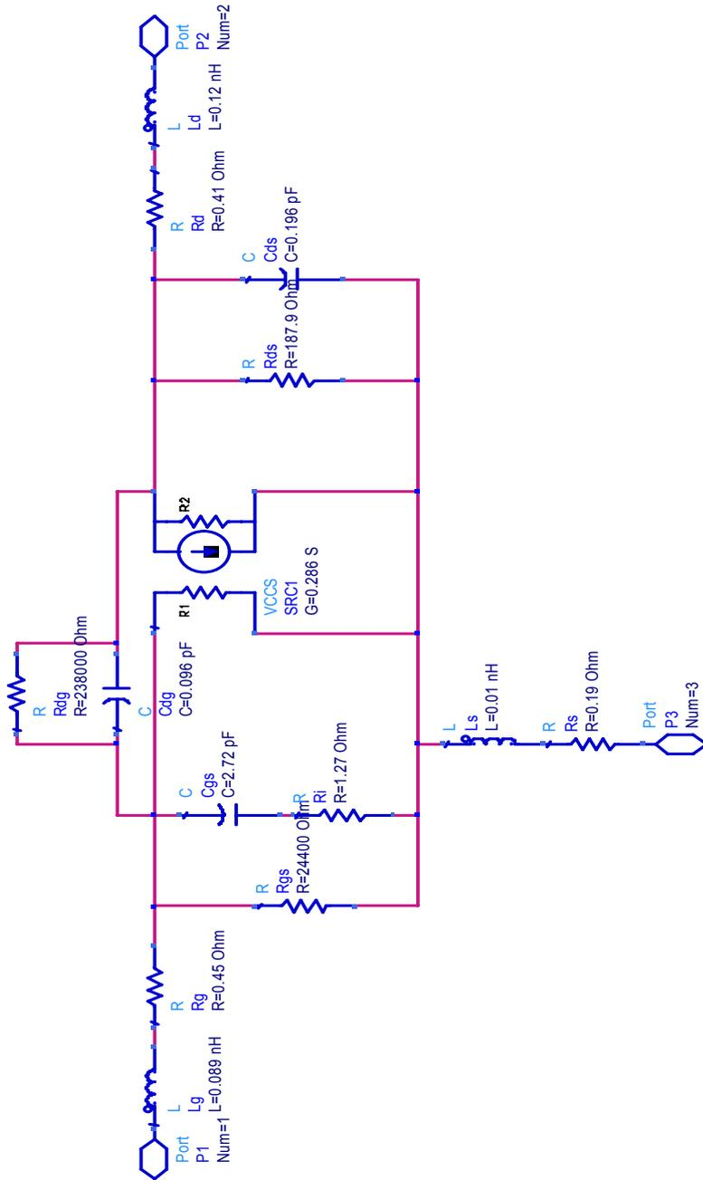
Figure 4-3: Linear Model of TGF2021-01 @  $V_d=12V$ ,  $I_{dq}=75mA$
