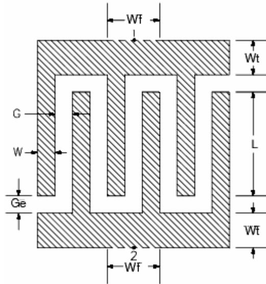
Figure 3-42: Layout of a Typical Microstrip Interdigital Capacitor
