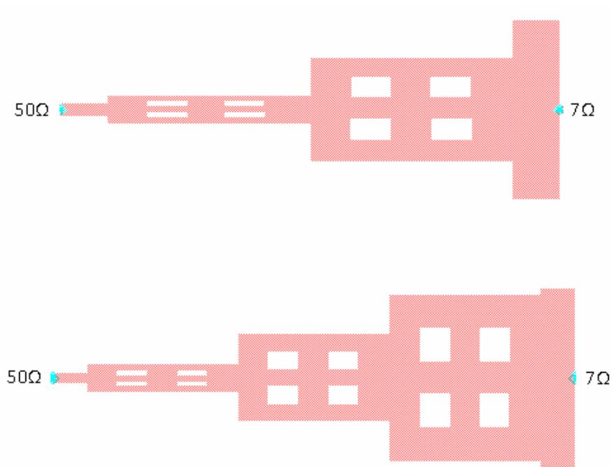
Figure 3-59: Layout of Matching Sections with Sierpinski Square for Iteration Order-1
