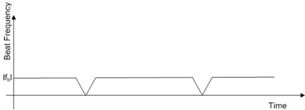
Figure 2-5: The beat frequency of triangular modulated signal
