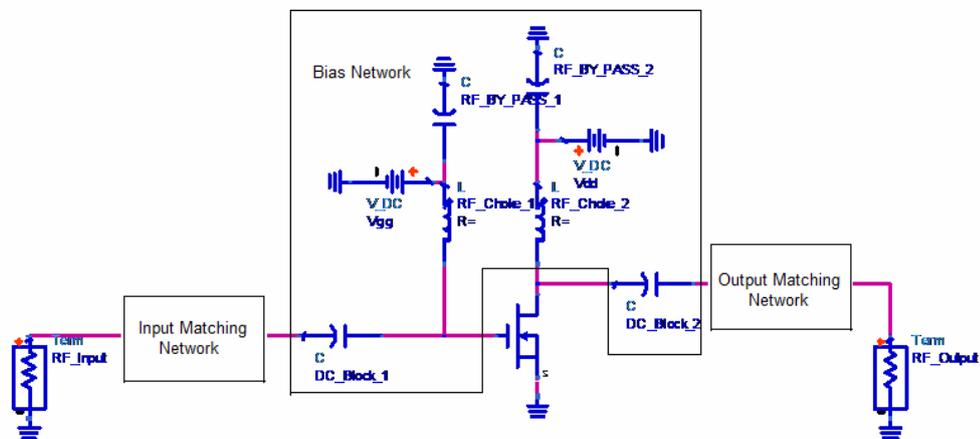
Figure 4-2: A Typical Single Stage Amplifier Schematic
