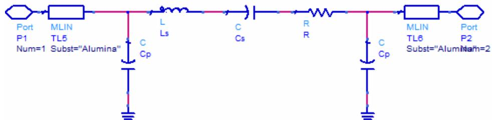
Figure 3-44: Lumped Element Equivalent Circuit of Interdigital Capacitor
