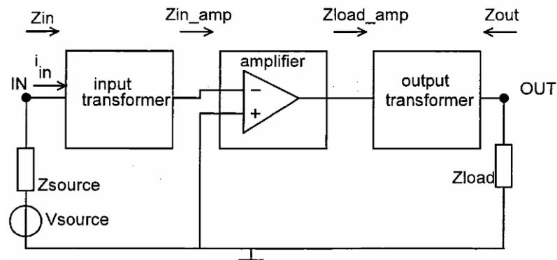
Figure 4-16: LNA with Input and Output Transformers
