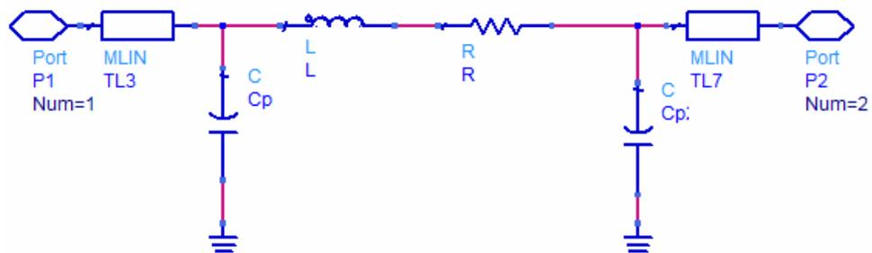
Figure 3-52: Equivalent Circuit for Rectangular Spiral Inductor
