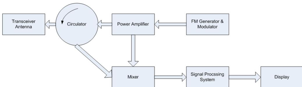
Figure 2-2: Basic block diagram of FMCW radar with one antenna
