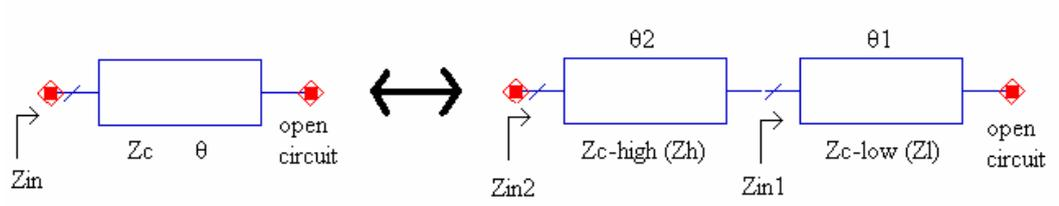
Figure 3-23: Schematic of Proposed Method for Quarter Wavelength Stub
