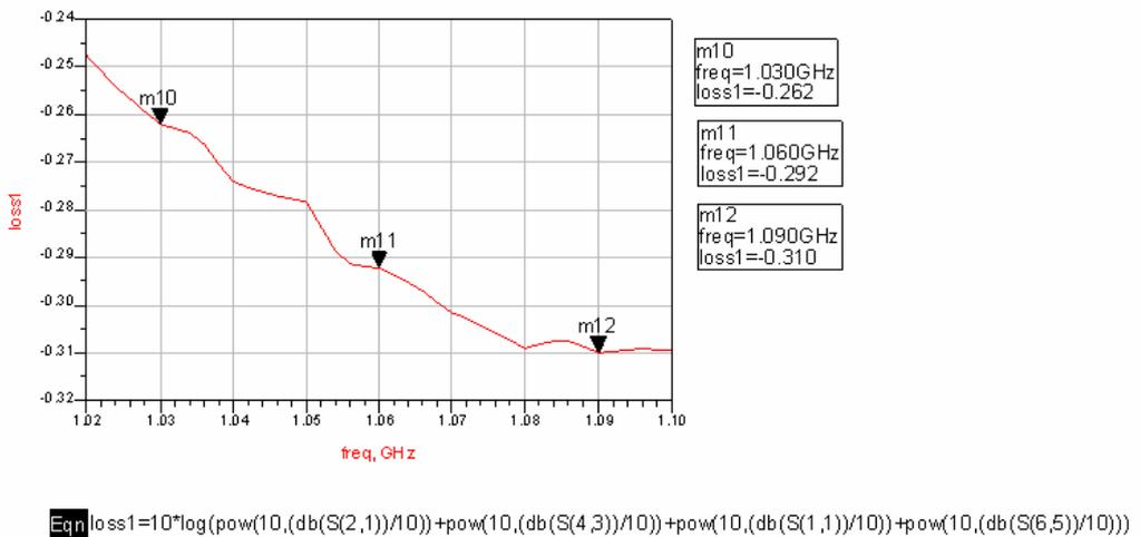
Figure 3-10: Total Loss of Dual Transmission Line Branch-Line Coupler
