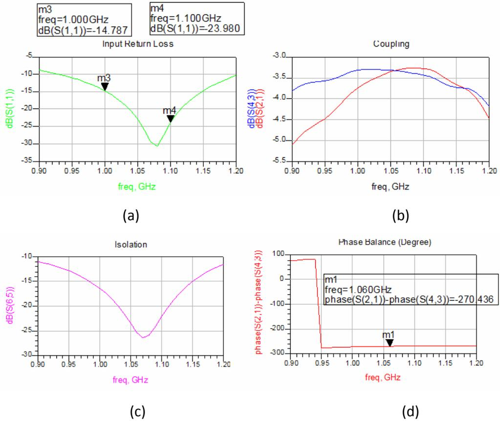
Figure 3-9: Measurement Results of Dual Transmission Line Branch-Line Coupler
