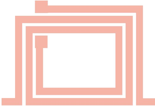
Figure 4-7: Layout of 2 <sup>3</sup>/<sub>4</sub> Turn Spiral Inductor
