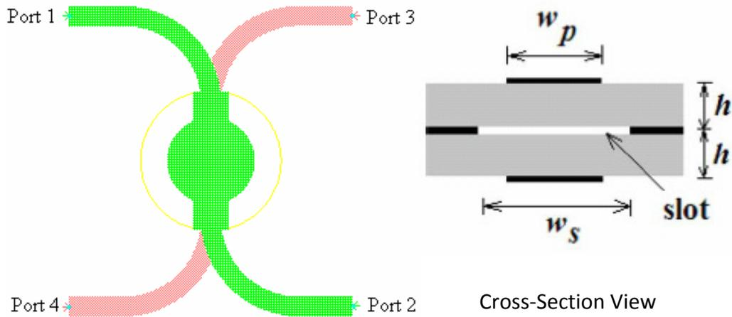
Figure 3-18: Simulated Layout of Aperture Coupled Directional Coupler
