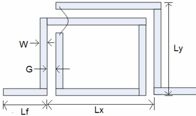
Figure 3-51: Layout of 1  $\frac{3}{4}$  Turn Rectangular Inductor
