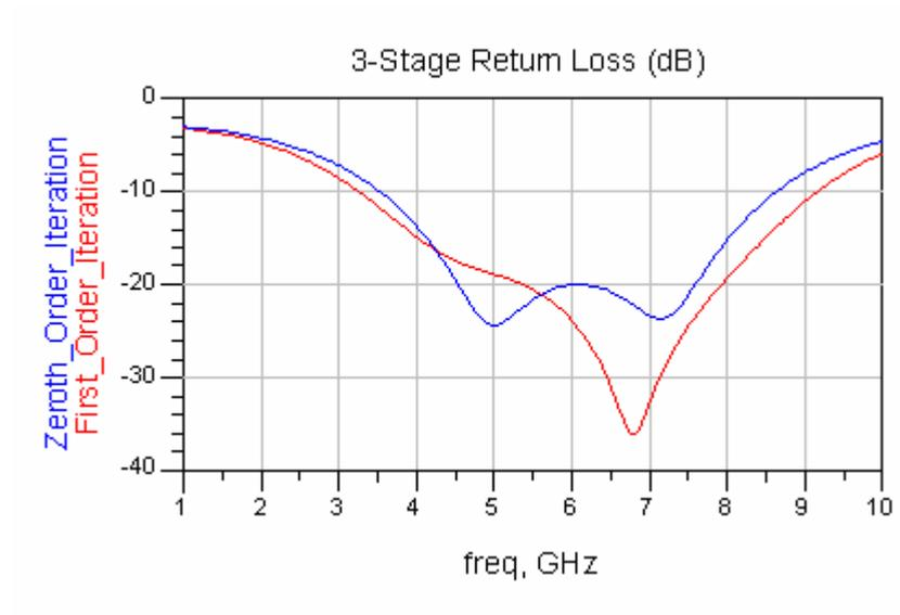
Figure 3-61: EM Simulation Result of 3-stage Matching Section Design
