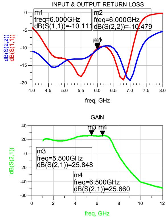
Figure 4-15: Simulation Results of Two Cascaded TGF2021-01 Amplifier
