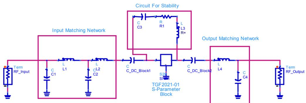
Figure 4-4: TGF2021-01 Input & Output Match with Ideal Components
