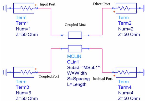
Figure 3-2: Schematic of a Coupled Line Coupler
