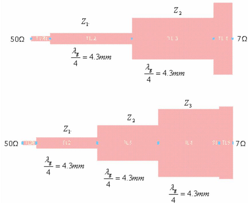
Figure 3-58: Layout of 2 and 3 Stage Matching Sections
