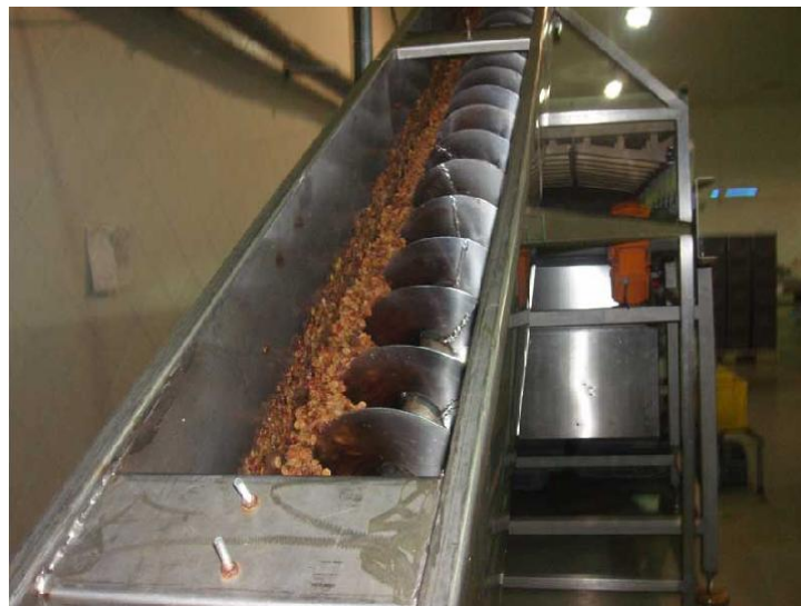
Figure 3.2: An application of a spiral conveying
