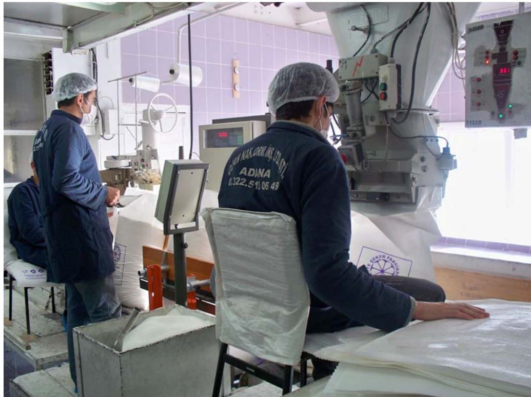
Figure 1.3: Weighing and bagging operation
