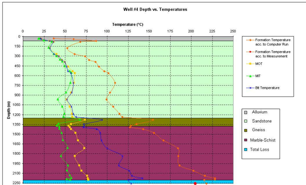
**Figure 7.4. Temperatures vs. Depth Graph of Well #4 for Case 1.**
