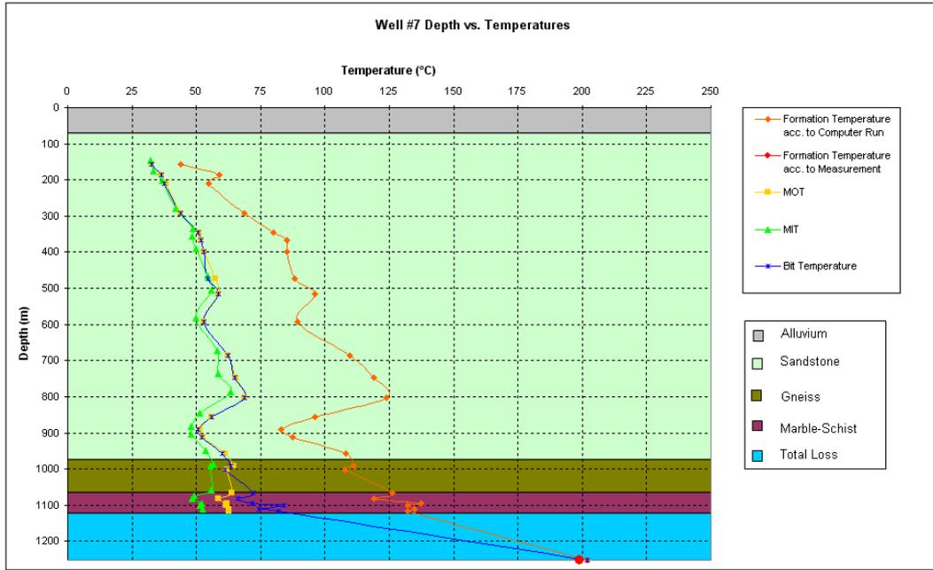
**Figure 7.11. Temperatures vs. Depth Graph of Well #7 for Case 2.**
