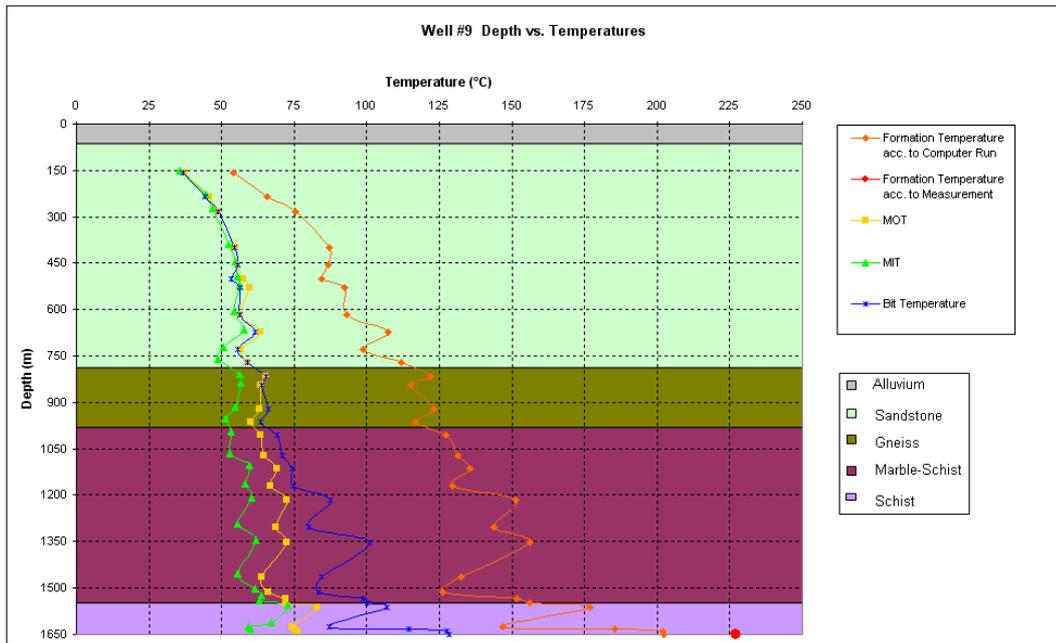
**Figure 7.14. Temperatures vs. Depth Graph of Well #9 for Case 2.**
