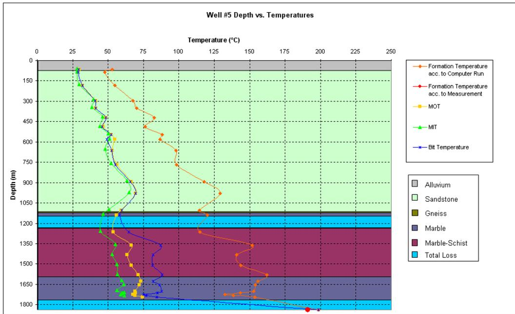
**Figure 7.8. Temperatures vs. Depth Graph of Well #5 for Case 2.**
