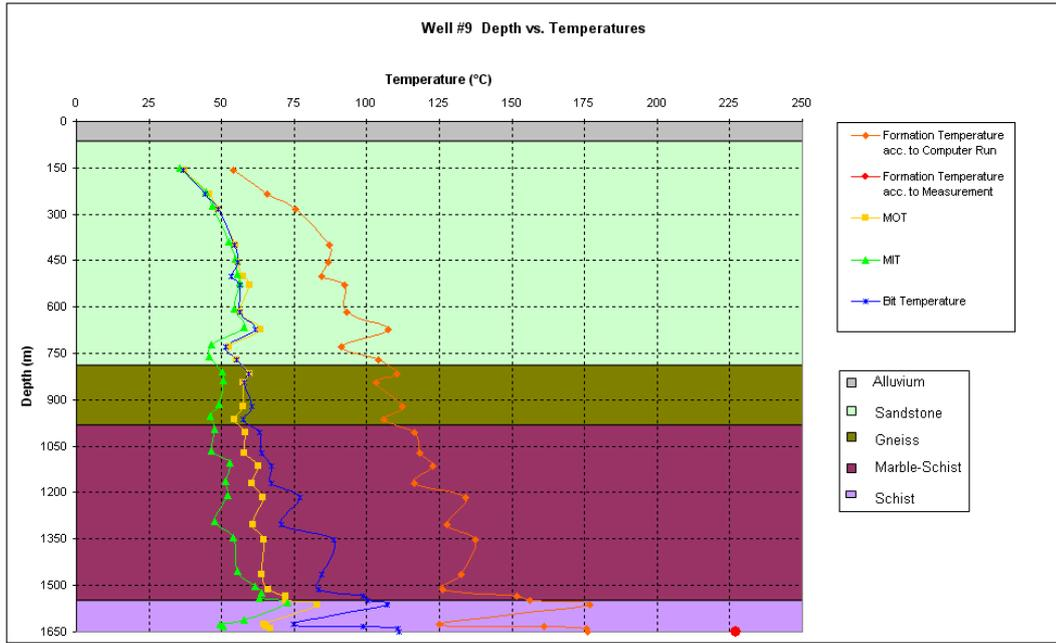
**Figure 7.13. Temperatures vs. Depth Graph of Well #9 for Case 1.**
