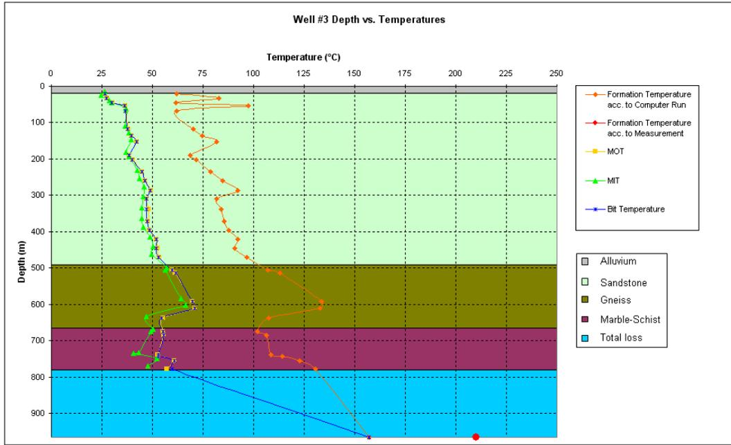
**Figure 7.1. Temperatures vs. Depth Graph of Well #3 for Case 1.**
