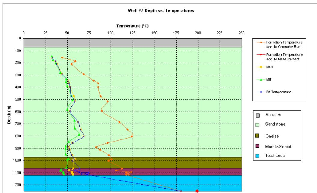
**Figure 7.10. Temperatures vs. Depth Graph of Well #7 for Case 1.**
