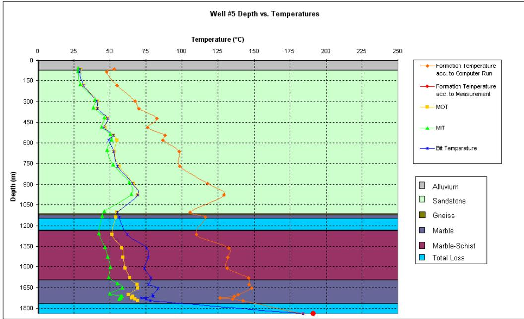
**Figure 7.7. Temperatures vs. Depth Graph of Well #5 for Case 1.**
