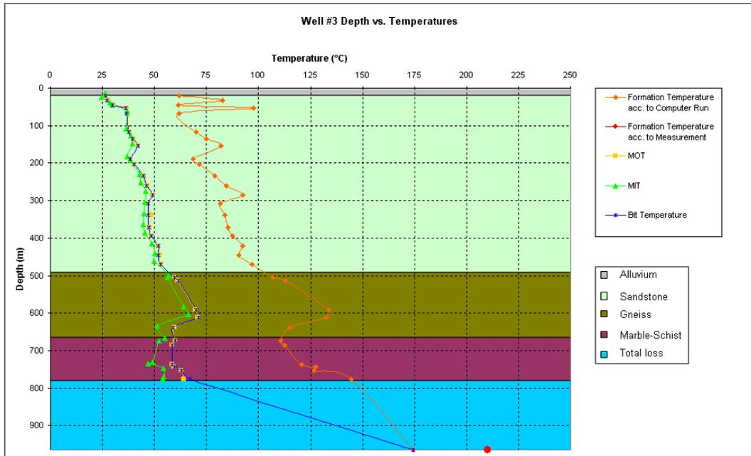
**Figure 7.2. Temperatures vs. Depth Graph of Well #3 for Case 2.**
