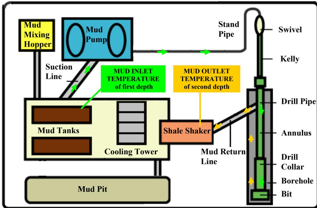
**Figure 6.1. Mud Inlet and Outlet Temperatures and Their Measurement Places in the Circulation System**
