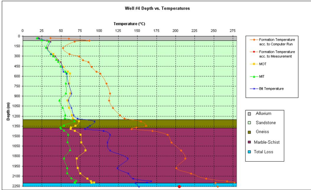
**Figure 7.5. Temperatures vs. Depth Graph of Well #4 for Case 2.**
