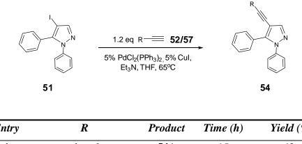
**Table 4.** Synthesis of 4-alkynyl-1,5-diphenyl-1*H*-pyrazoles (54A-E).
