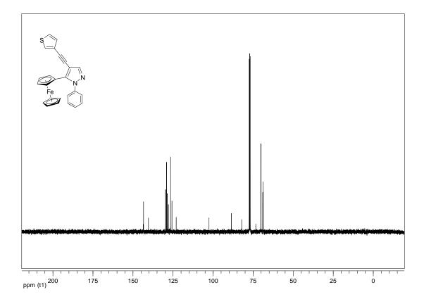
Figure A12. <sup>13</sup>C NMR spectra of 53F.
