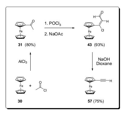
Figure 29. Synthesis of acetylferrocene (31), (2-formyl-1-chlorovinyl)ferrocene (43) and ethynylferrocene (57).
