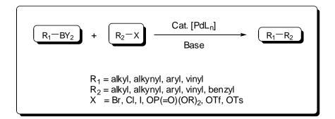
Figure 25. General scheme of Suzuki-Miyaura coupling reaction.
