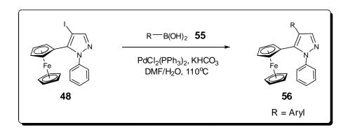
Figure 28. Synthesis of 4-aryl-5-ferrocenyl-1-phenyl-1*H*-pyrazoles (56).
