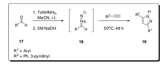
Figure 10. Synthesis of pyrazole derivatives by 1,3-dipolar cycloaddition of diazo compounds 18 with acetylenes.
