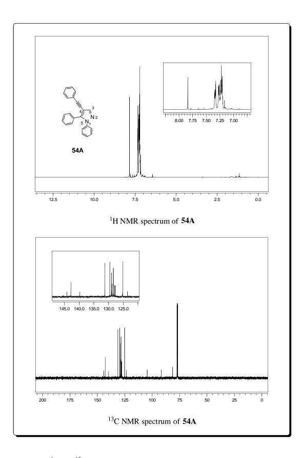
**Figure 41.** <sup>1</sup>H and <sup>13</sup>C NMR spectra of 1,5-diphenyl-4-(phenylethynyl)-1*H*-pyrazole (**54A**).
