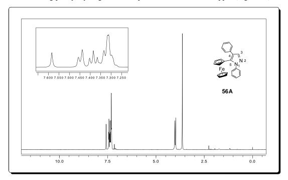
Figure 44. <sup>1</sup>H NMR spectrum of 5-ferrocenyl-1,4-diphenyl-1*H*-pyrazole (56A).
