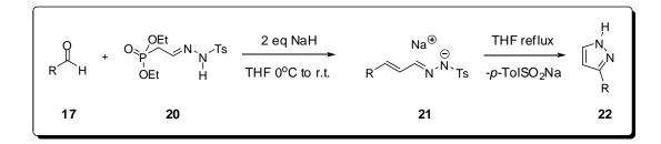
Figure 11. Synthesis of 3-(5)-substituted pyrazoles 22 by a [1 + 4] approach from aldehydes 17 and diethoxyphosphorylacetaldehyde tosylhydrazone (20).
