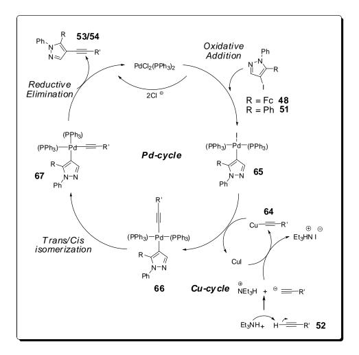
Figure 47. Mechanism of Sonogashira coupling reaction.
