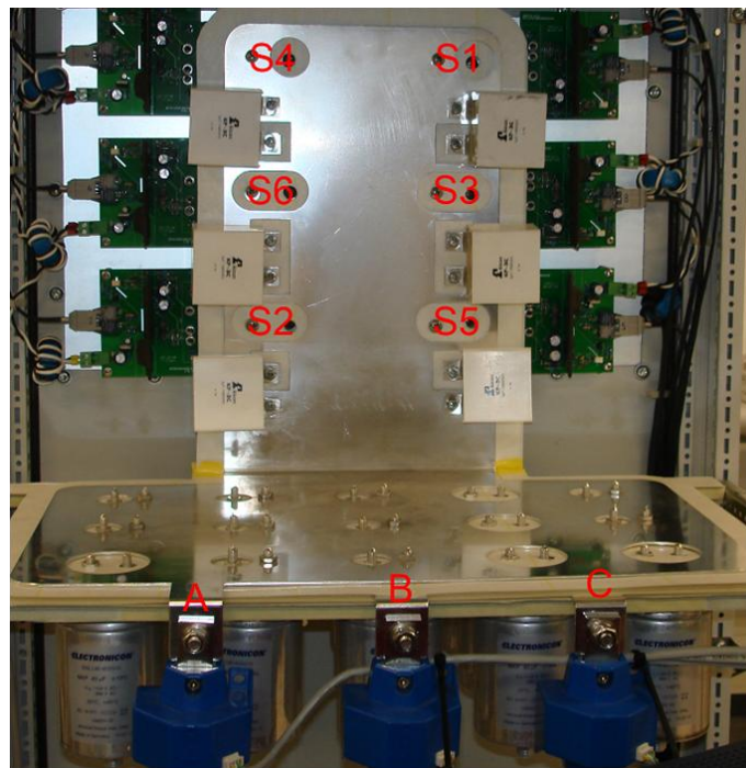
Figure 3.18 Power Stage of CSC STATCOM
