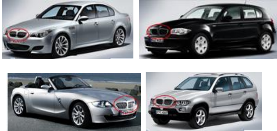
Figure 2.4 The kidney-shape grill as an artificial design feature used steadily over the product portfolio. (BMW homepage: www.bmw.com.tr )
