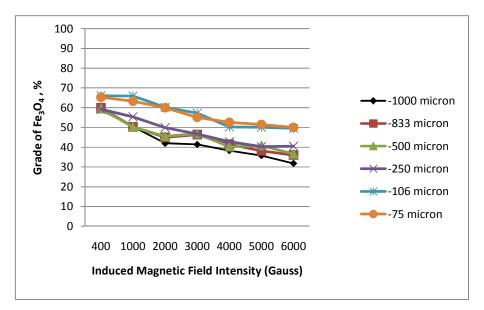
Figure 4.8 Grade of Fe3O4% versus magnetic field intensity for low grade tailing
