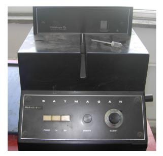
Figure 3.1 Satmagan (saturation magnetic analyzer)
