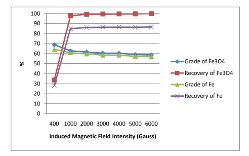
Figure 4.17 Results of the magnetic concentration test for -1000 micron material (App. C, Table C.1)
