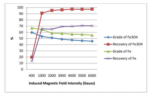
Figure 4.11 Results of the magnetic concentration test for -500 micron material (App. B, Table B.3)
