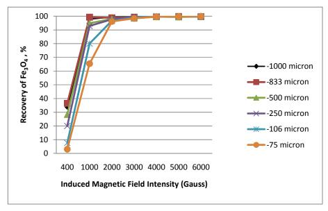
Figure 4.23 Recovery of  $Fe_3O_4\%$  versus magnetic field intensity for high grade tailing
