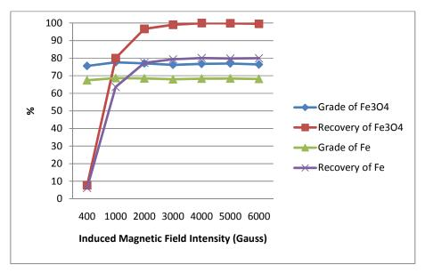
Figure 4.21 Results of the magnetic concentration test for -106 micron material (App. C, Table C.5)
