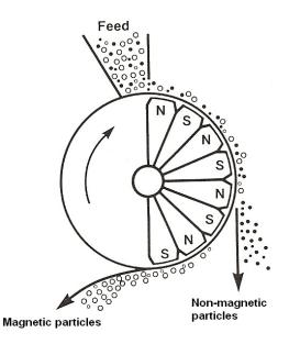
Figure 2.13 Low intensity dry drum type magnetic separator (Svoboda, 1987)
