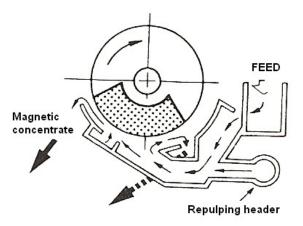
Figure 2.16 Counter-current magnetic separator (Svoboda, 1987)
