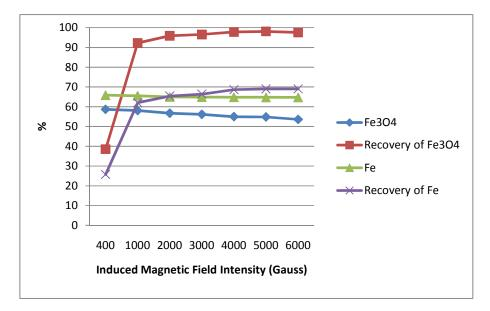
Figure 4.12 Results of the magnetic concentration test for -250 micron material (App. B, Table B.4)
