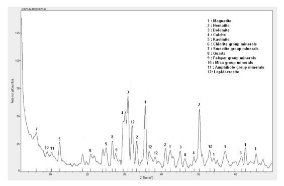
Figure 3.11 XRD pattern of medium grade tailing
