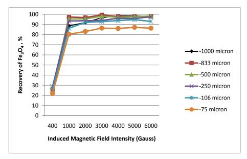
Figure 4.7 Recovery of Fe3O4% versus magnetic field intensity for low grade tailing
