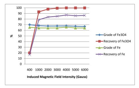
Figure 4.20 Results of the magnetic concentration test for -250 micron material (App. C, Table C.4)
