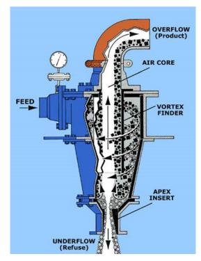
Figure 2.10 Water-only cyclone (www.flsmidthminerals.com)
