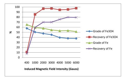
Figure 4.9 Results of the magnetic concentration test for -1000 micron material (App. B, Table B.1)
