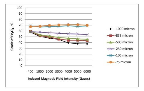
Figure 4.16 Grade of  $Fe_3O_4\%$  versus magnetic field intensity for medium grade tailing
