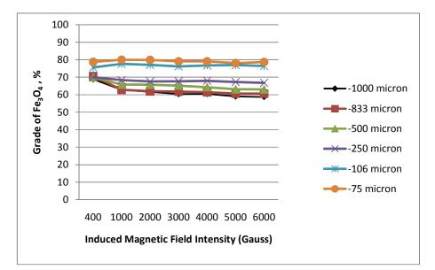
Figure 4.24 Grade of  $Fe_3O_4\%$  versus magnetic field intensity for high grade tailing
