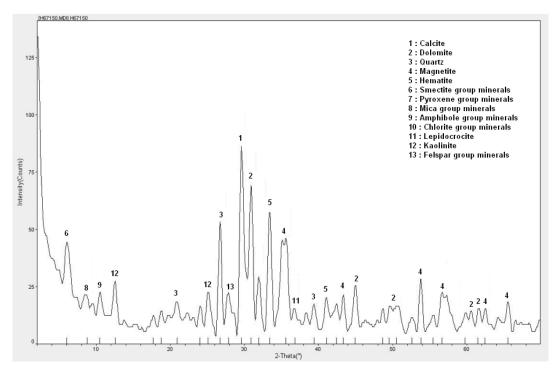
Figure 3.12 XRD pattern of low grade tailing
