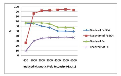
Figure 4.5 Results of the magnetic concentration test for -106 micron material (App. A, Table A.5)
