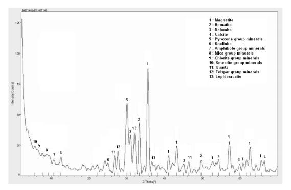
Figure 3.10 XRD pattern of high grade tailing
