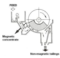
Figure 2.15 Counter-rotation magnetic separator (Svoboda, 1987)
