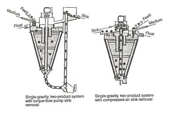
Figure 2.3 Cone separator
