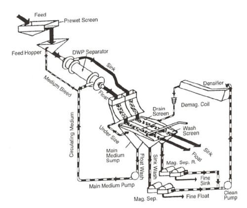
Figure 2.11 HMS circuit with regeneration unit (Wills, 1985)
