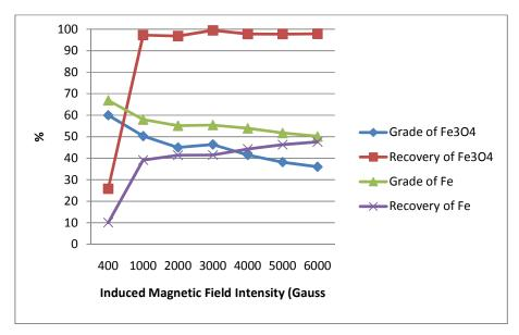
Figure 4.2 Results of the magnetic concentration test for -833 micron material (App. A, Table A.2)
