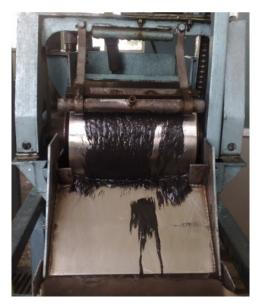
Figure 4.25 Low intensity wet magnetic drum separator
