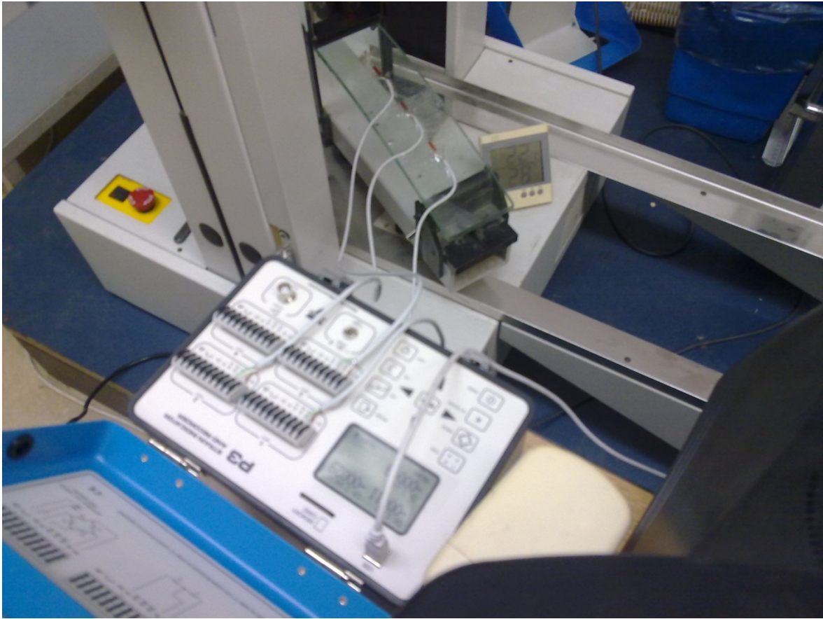
Figure 3.4. 3-point bending setup for laminated glass beam.
