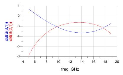
Figure 4.113 S21 and S31 of 6-18 GHz Lange coupler.
