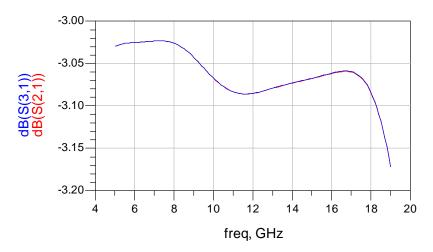
Figure 4.110 S21 and S31of 6-18 GHz power divider.
