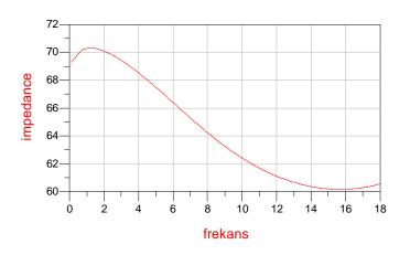
Figure 4.9 Diode impedance vs. frequency.
