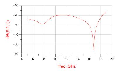
Figure 4.111 S11 of 6-18 GHz power divider.
