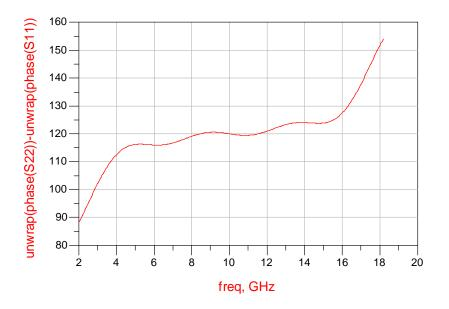
Figure 3.50 Differential phase response of the short circuited phase shifter branch 1.
