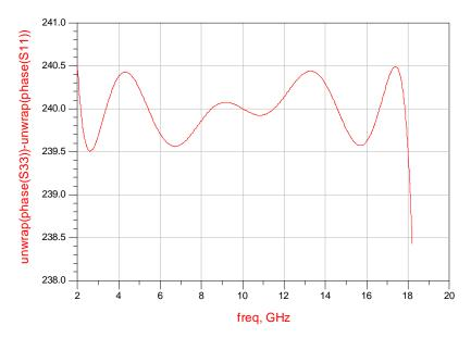
Figure 3.60 Differential phase response of final phase shifter structure for phase shifter branch 1
