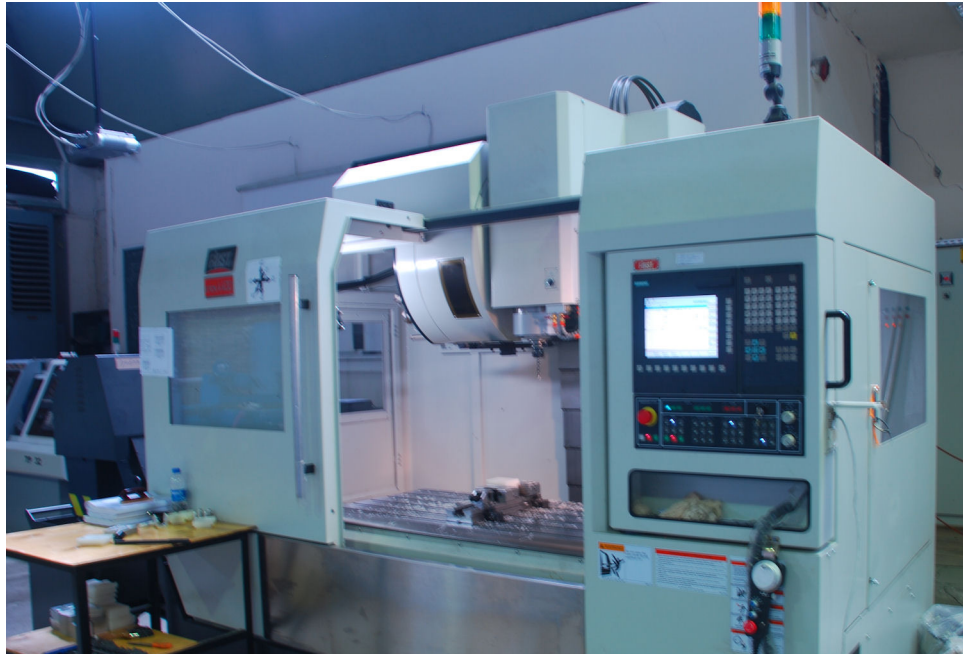
Figure 6.6: First MCV-1100 3-Axis CNC Machining Center
