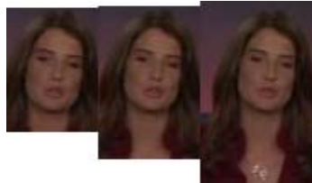
Figure 2.2. A problem with CamShift. The face rectangle grows rapidly due to skin colored pixels in the neck region.
