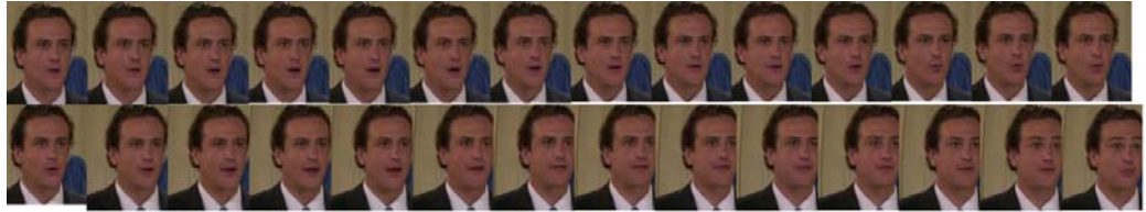
Figure 2.3. Output of the particle filter face tracker. Faces are not centered. There is a significant amount of background clutter.
