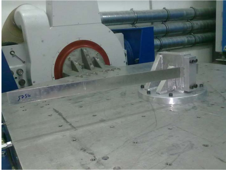
Figure 5.17 – Damaged specimen 1: without mean stress
