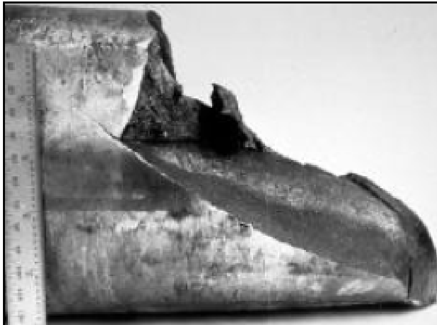
Figure 1.3 –A fatigue failure surface [52]
