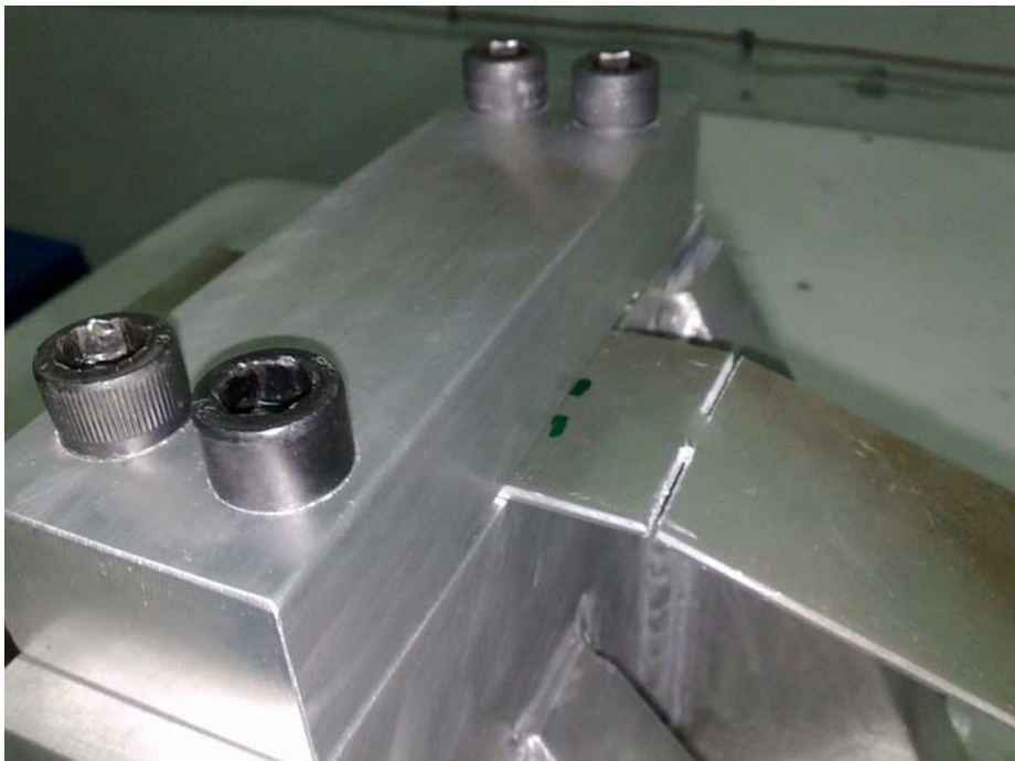
Figure 5.20 – Damaged specimen 2: with mean stress (close-up)
