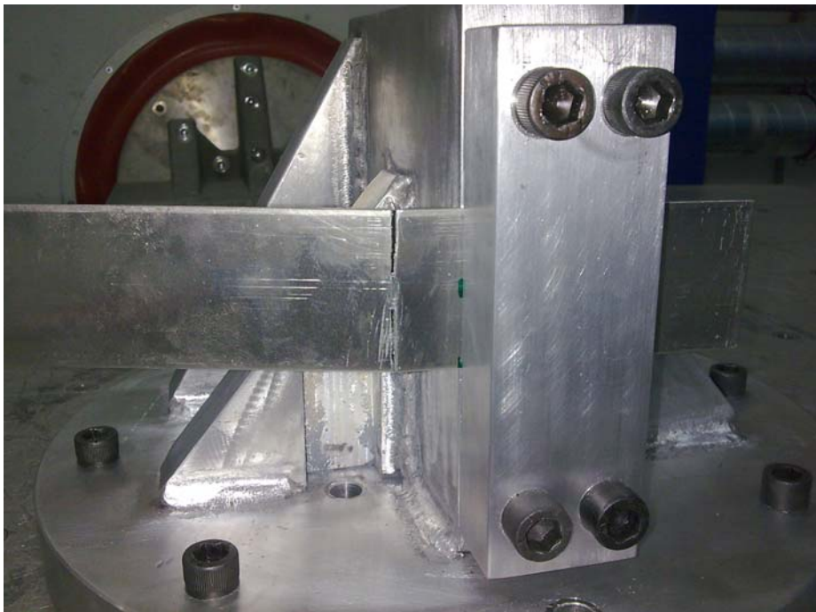
Figure 5.22 – Damaged specimen 3: with proposed method (close-up)
