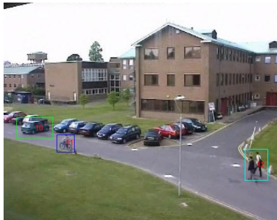
Figure 4-24 An example from test video3 – Tracking of multiple targets labeled as 10, 11 and 12
