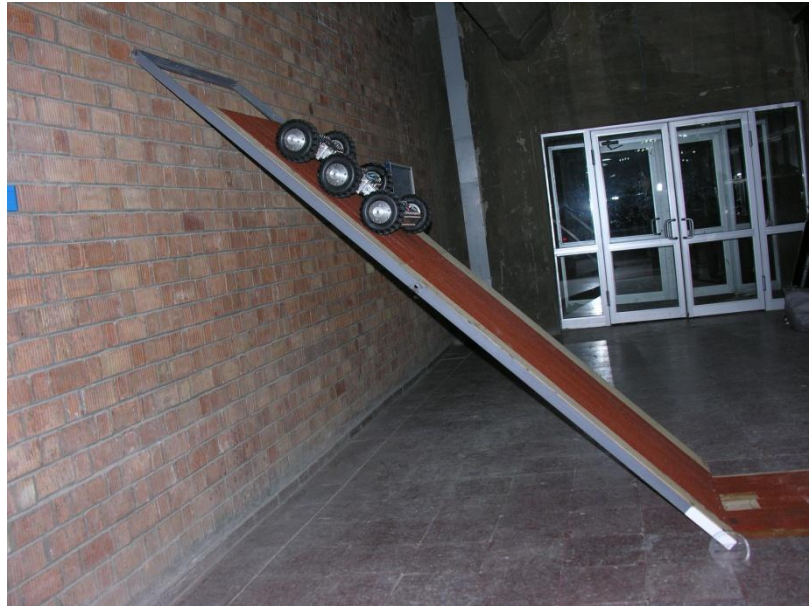
Figure 42 Robot climbing a slope experiment setup
