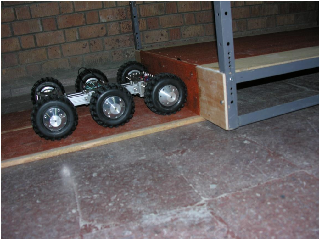
Figure 46 Robot platform going over a step experiment setup
