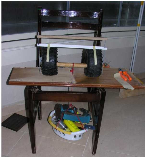
Figure 23 Wheel stiffness measurement test platform
