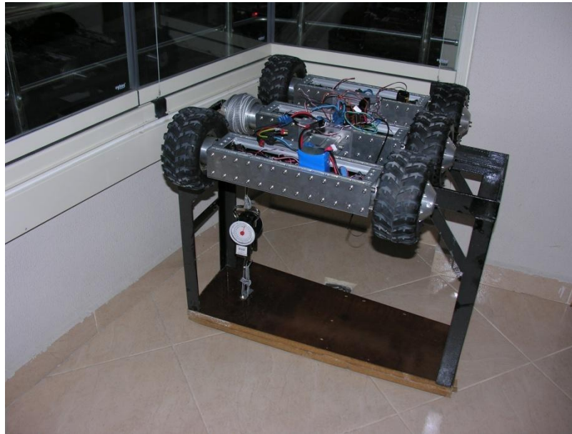
Figure 40 Stall torque measurement experiment setup
