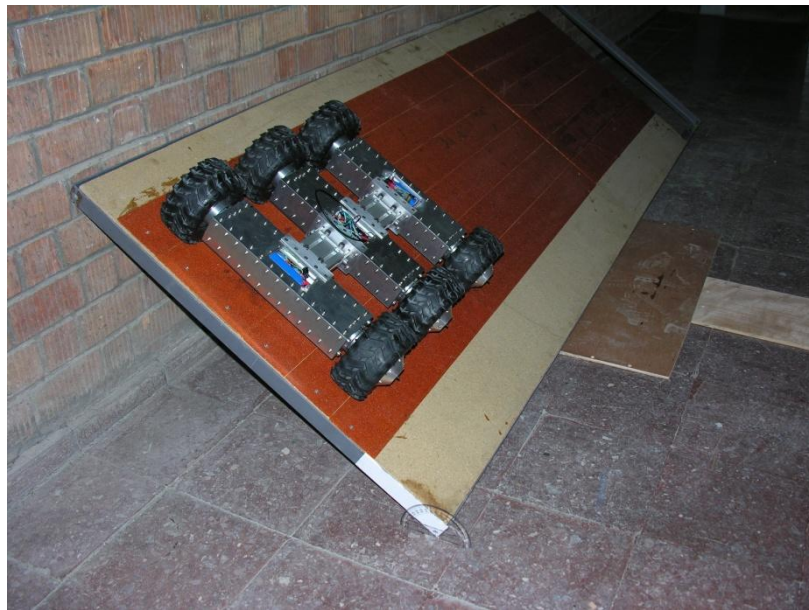
Figure 44 Robot platform going at an inclined surface experiment setup
