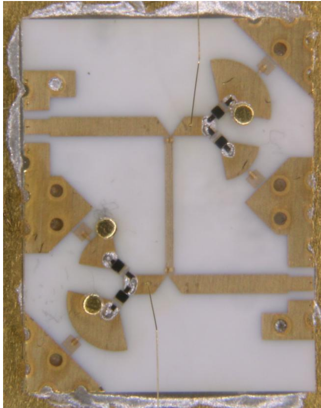
Figure 7.18 Close View of Fabricated 45^\circ Phase Shifter with Spiral Inductors.
