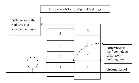
Figure 5.25 Hammering Impacts of Adjacent Buildings in the Earthquake
