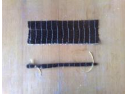
Figure 4.18 General views of FRP anchorage and the wrapped FRP sheet.
