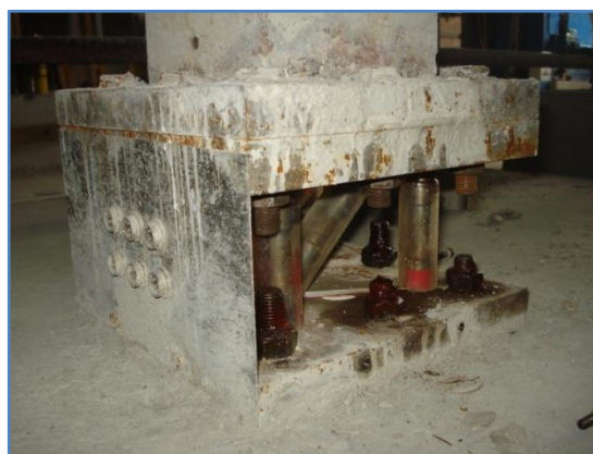
Figure 4.7 General view of the force transducers.
